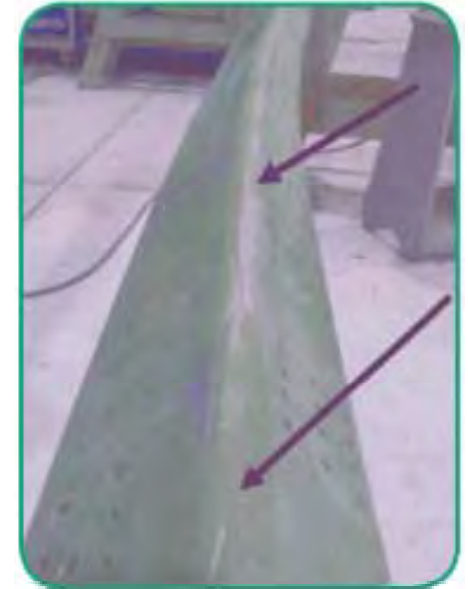
Arrows indicate crack in attach angle
