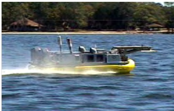
Fig. 3. 1/6th-scale free-running LCAC model in Panama City, Florida
