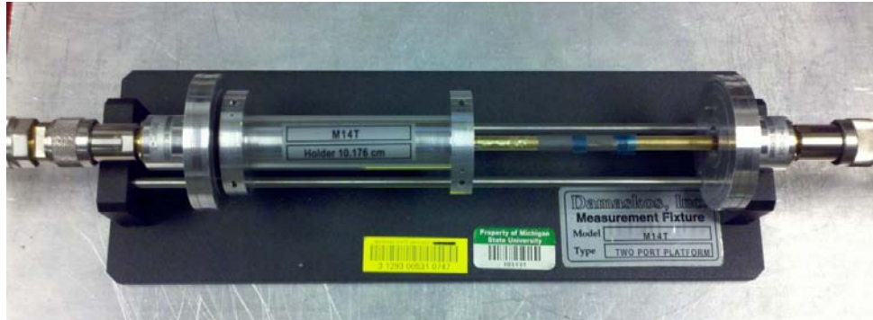
Figure 4.1: Coaxial Test Fixture with Sample Holder and Inner Conductor Exposed
