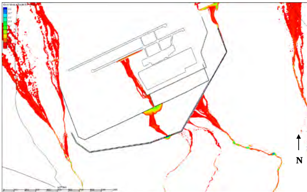
Figure 57. Alternative 2-B inundation depths, at 7.5 hours, m.
