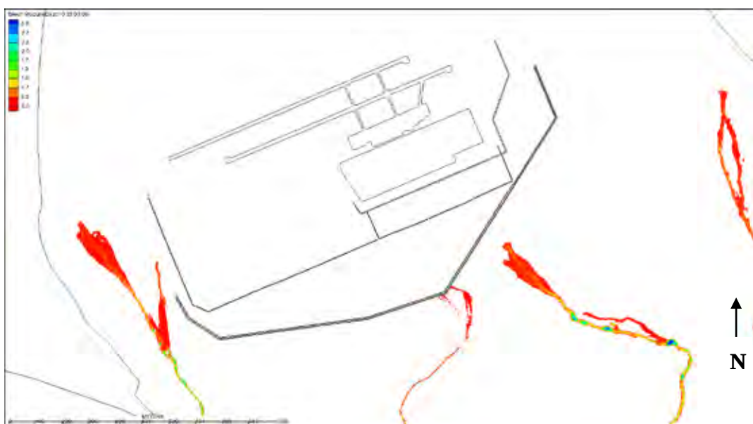
Figure 53. Alternative 2-B inundation depths, at 3 hours, m.
