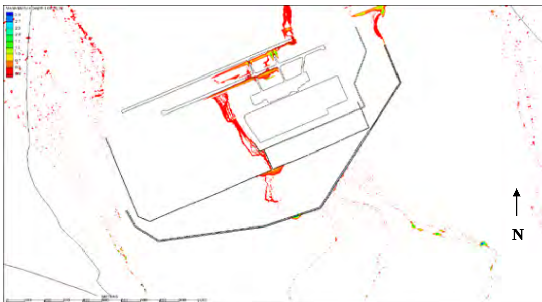
Figure 59. Alternative 2-B inundation depths, at 24 hours, m.
