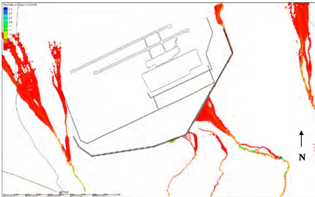
Figure 55. Alternative 2-B inundation depths, at 4 hours, m.
