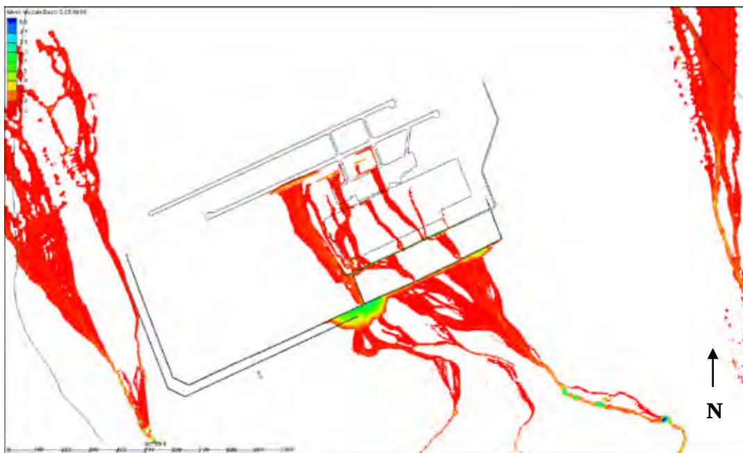
Figure 46. Alternative 1-B inundation depths, at 5 hours, m.
