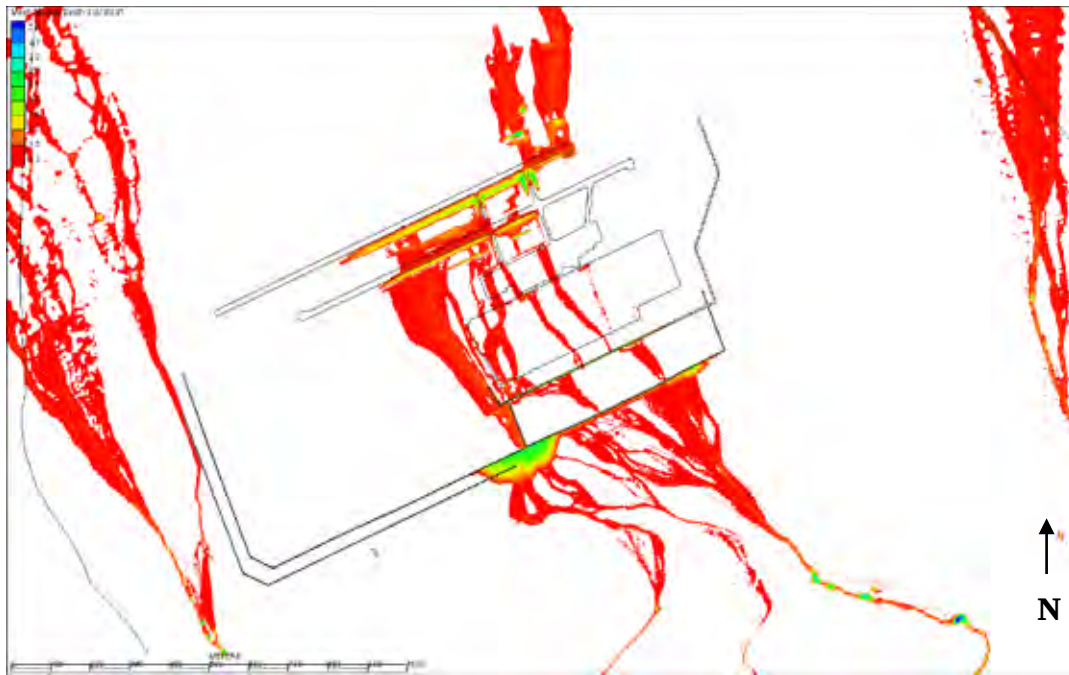
Figure 47. Alternative 1-B inundation depths, at 7.5 hours, m.
