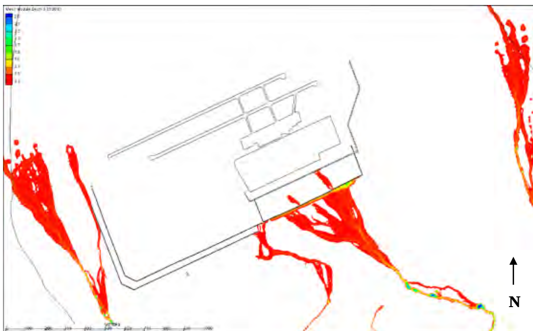
Figure 44. Alternative 1-B inundation depths, at 3.5 hours, m.
