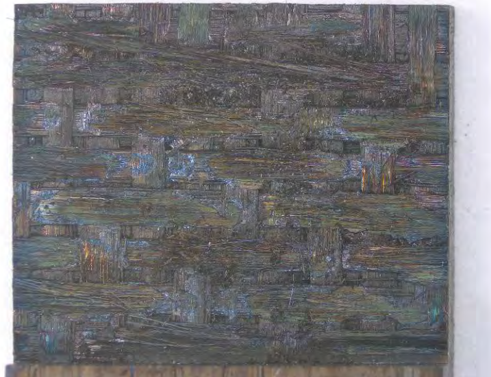
Figure 91 – P8-1, Fracture surface of Hi-Nicalon/PyC/HyperSiC Ceramic Composite specimen tested in compression to failure at 1200 °C in air
