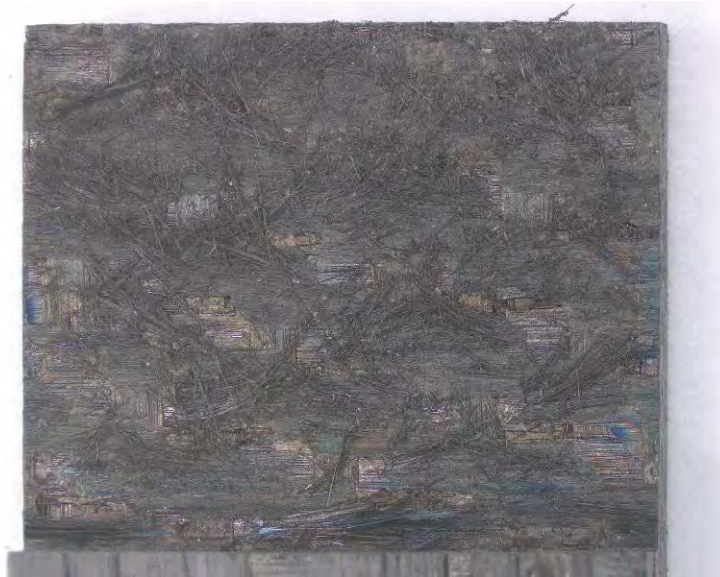
Figure 44 – P9-3, Fracture surface of Hi-Nicalon/PyC/HyperSiC Ceramic Composite specimen tested in creep at -20 MPa and 1200 °C in steam
