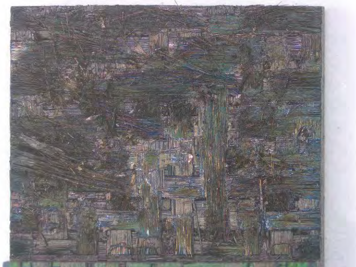
Figure 101 – P9-4, Fracture surface of Hi-Nicalon/PyC/HyperSiC Ceramic Composite specimen tested in creep at -22 MPa and 1200 °C in steam
