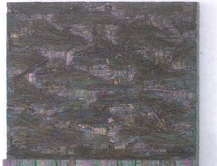
Figure 95 – P9-2, Fracture surface of Hi-Nicalon/PyC/HyperSiC Ceramic Composite specimen tested in creep at -18 MPa and 1200 °C in air
