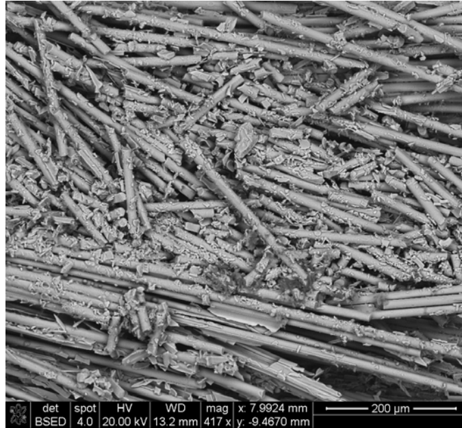
Figure 76 - SEM image showing fractured fibers bound with glass and matrix of Hi-Nicalon/PyC/HyperSiC Ceramic Composite specimen tested in compression at 20 MPa at 1200 °C in steam
