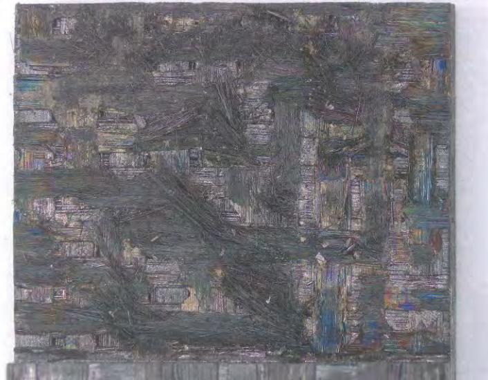
Figure 43 – P8-5, Fracture surface of Hi-Nicalon/PyC/HyperSiC Ceramic Composite specimen tested in creep at -18 MPa and 1200 °C in steam
