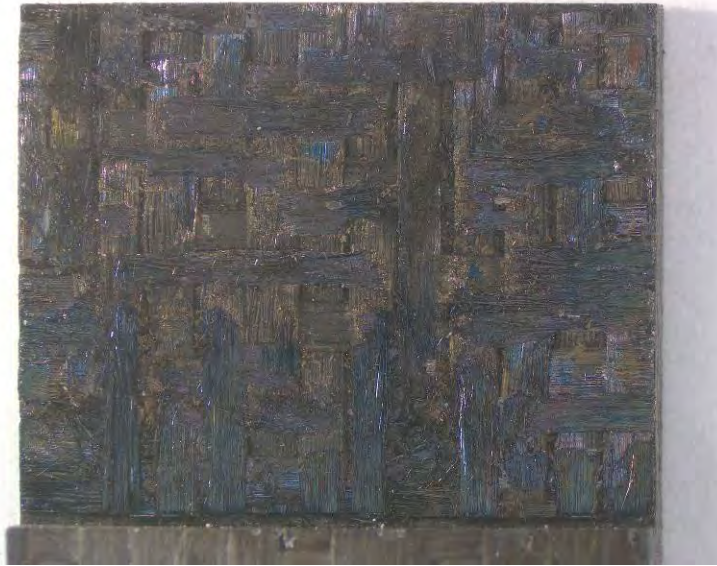
Figure 34 – P6-3, Fracture surface of Hi-Nicalon/PyC/HyperSiC Ceramic Composite specimen tested in compression to failure at 1200 °C in air
