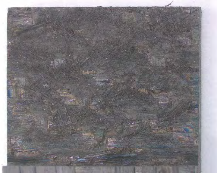
Figure 100 – P9-3, Fracture surface of Hi-Nicalon/PyC/HyperSiC Ceramic Composite specimen tested in creep at -20 MPa and 1200 °C in steam
