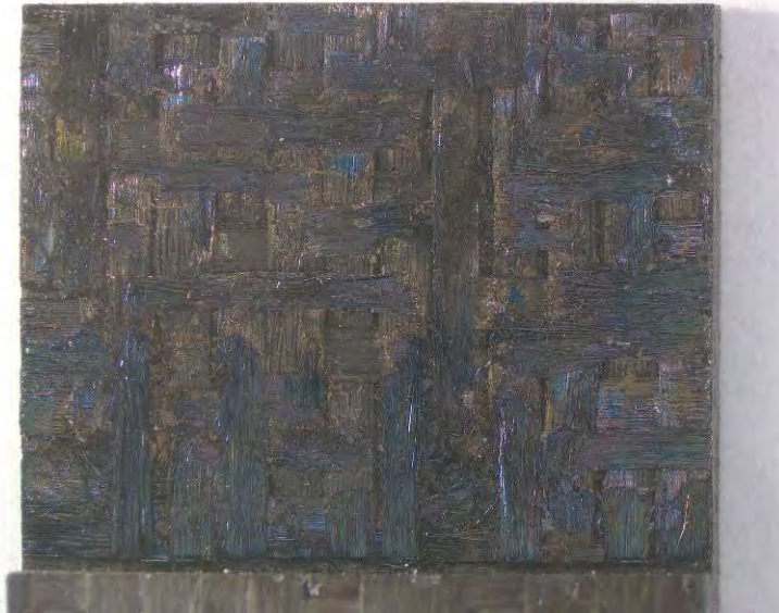
Figure 90 – P6-3, Fracture surface of Hi-Nicalon/PyC/HyperSiC Ceramic Composite specimen tested in compression to failure at 1200 °C in air
