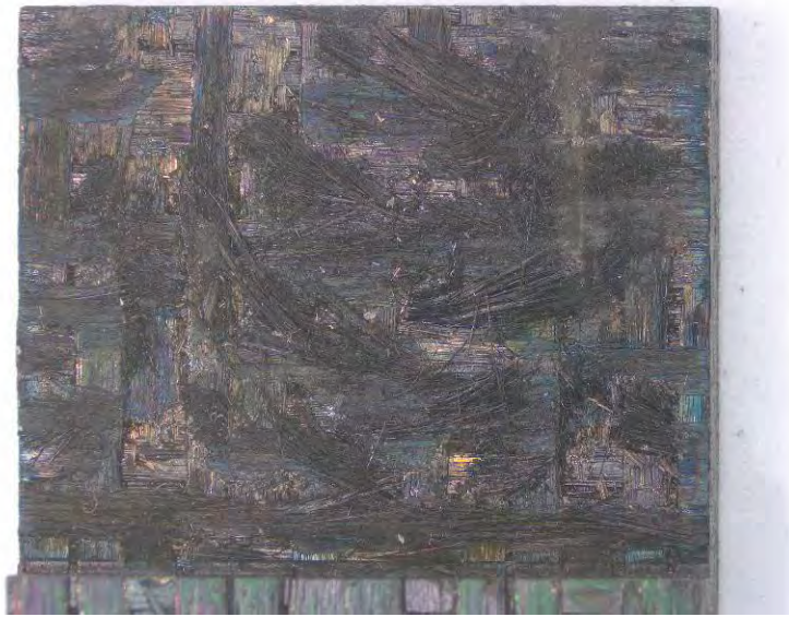
Figure 94 – P6-4, Fracture surface of Hi-Nicalon/PyC/HyperSiC Ceramic Composite specimen tested in creep at -16 MPa and 1200 °C in air
