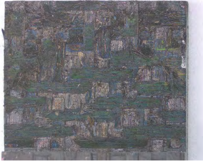
Figure 42 – P2-5, Fracture surface of Hi-Nicalon/PyC/HyperSiC Ceramic Composite specimen tested in creep at -16 MPa and 1200 °C in steam
