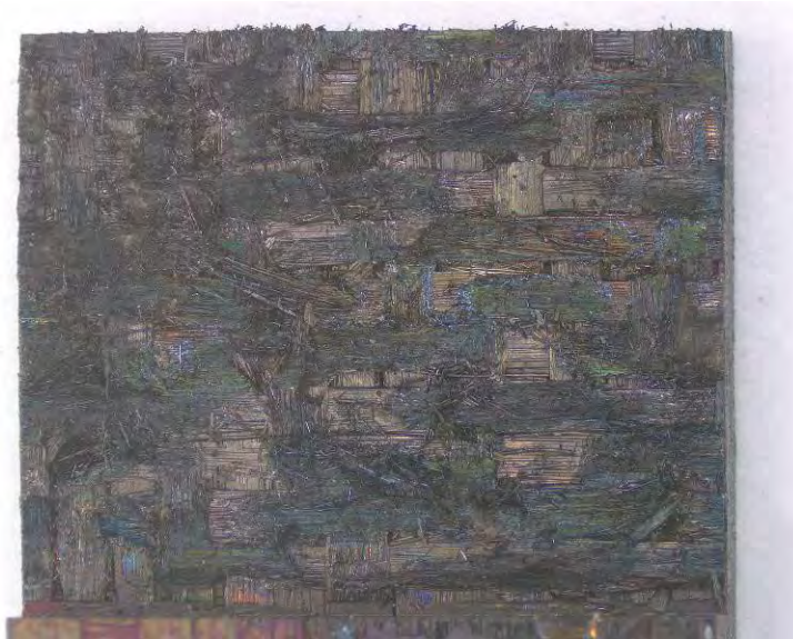
Figure 41 – P2-6, Fracture surface of Hi-Nicalon/PyC/HyperSiC Ceramic Composite specimen tested in creep at -22 MPa and 1200 °C in air
