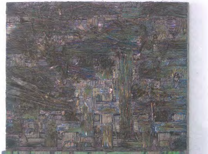
Figure 45 – P9-4, Fracture surface of Hi-Nicalon/PyC/HyperSiC Ceramic Composite specimen tested in creep at -22 MPa and 1200 °C in steam
