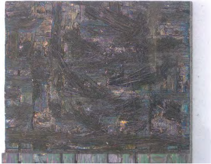
Figure 38 – P6-4, Fracture surface of Hi-Nicalon/PyC/HyperSiC Ceramic Composite specimen tested in creep at -16 MPa and 1200 °C in air
