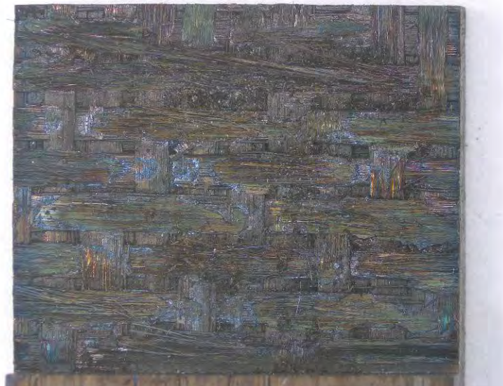
Figure 35 – P8-1, Fracture surface of Hi-Nicalon/PyC/HyperSiC Ceramic Composite specimen tested in compression to failure at 1200 °C in air
