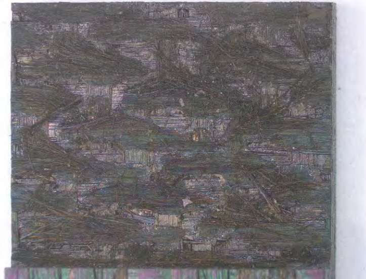
Figure 39 – P9-2, Fracture surface of Hi-Nicalon/PyC/HyperSiC Ceramic Composite specimen tested in creep at -18 MPa and 1200 °C in air
