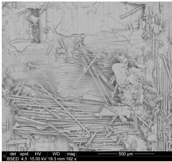
Figure 135 - SEM image showing delamination zone with debris of Hi-Nicalon/PyC/HyperSiC Ceramic Composite specimen tested in compression at 22 MPa at 1200 °C in air
