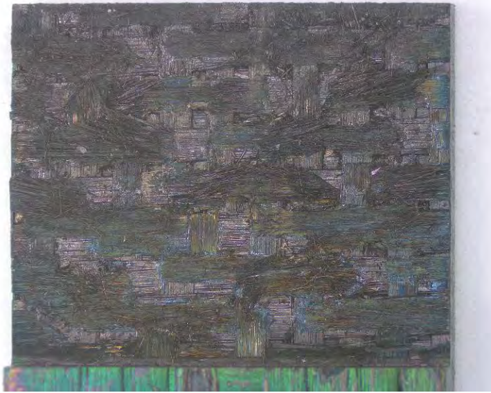
Figure 40 – P8-4, Fracture surface of Hi-Nicalon/PyC/HyperSiC Ceramic Composite specimen tested in creep at -20 MPa and 1200 °C in air
