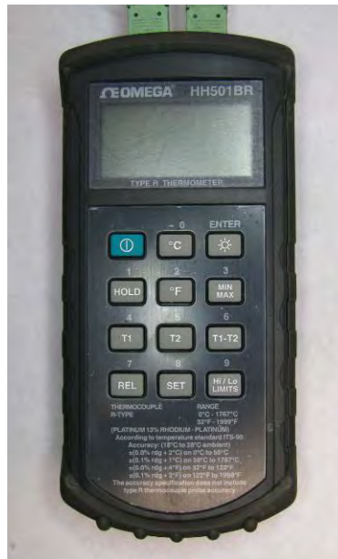
Figure 9 - Omega HH501BR thermometer
