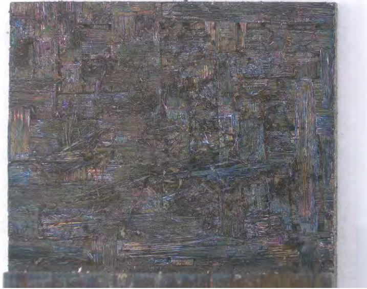
Figure 36 – P2-3, Fracture surface of Hi-Nicalon/PyC/HyperSiC Ceramic Composite specimen tested in compression to failure at 1200 °C in air
