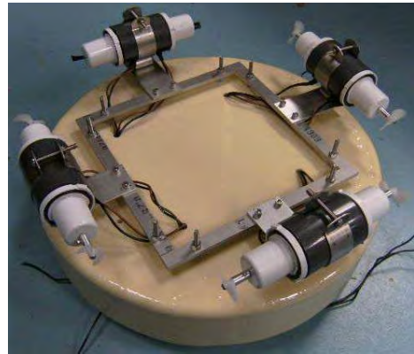
(b) Photograph of raft frame with attached motors
