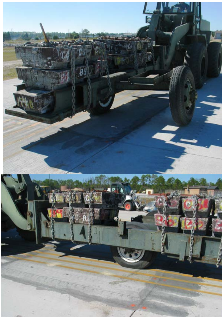
Figure 31. Accelerated Loading of the Repaired Sections Using F-15 Load Cart
