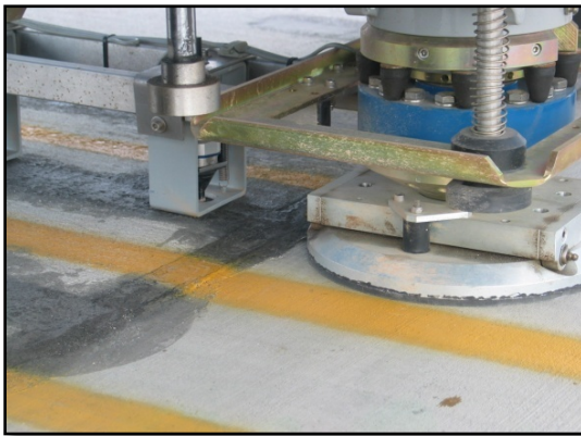
Figure 30. Placement of HWD Loading Frame and Geophones at the Edge of the Slabs
