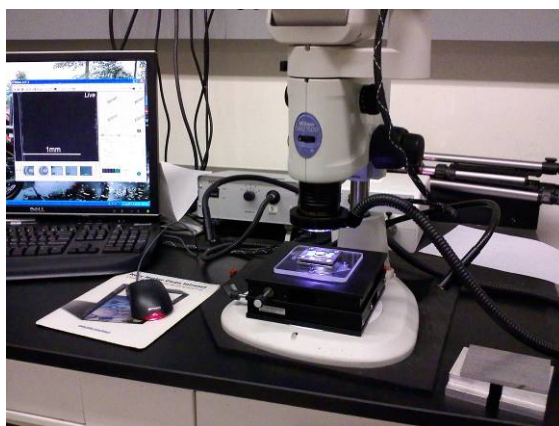
Figure 4-12. Diffusion cell experiment set-up
