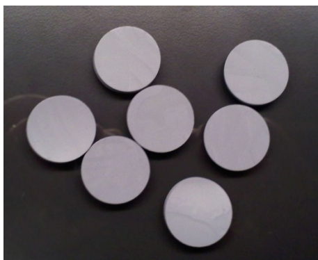
Figure 4-7. MIL-PRF-85285 fully formulated samples for gravimetric solvent sorption test
