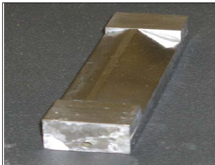
Figure 4-4: Byrd film applicator used for casting a thin film
