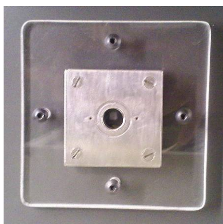
Figure 4-11. Top View of diffusion cell on acrylic plate
