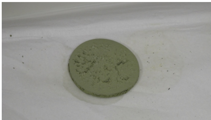
Figure 5-24. Surface degradation of MIL-PRF-23377 fully formulated sample exposed to MC/PhOH
