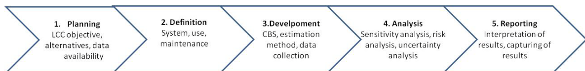
Figure 8 Steps in a Life Cycle Cost Analysis (Bassford, Voort, Boer, & Pung, 2008)
