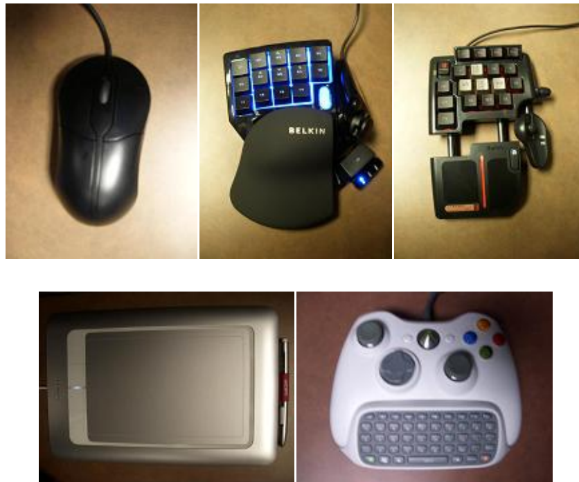
Figure 1. Control devices used in the study. Upper row (left to right): standard mouse, Belkin n52te, and Saitek Cyborg Command Unit; lower row (left to right): Wacom Bamboo Fun (with stylus or touch) and Xbox 360 controller.
