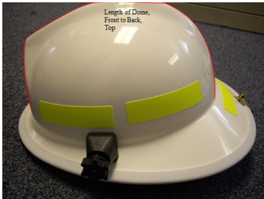
Figure 11. Schematic Showing Measurement of Dome from Front to Back
