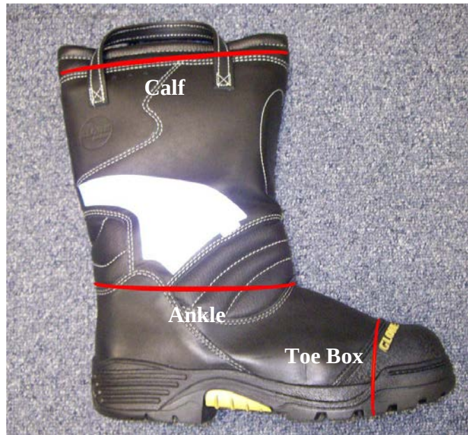
Figure 14. Schematic Showing Boot Measurements
