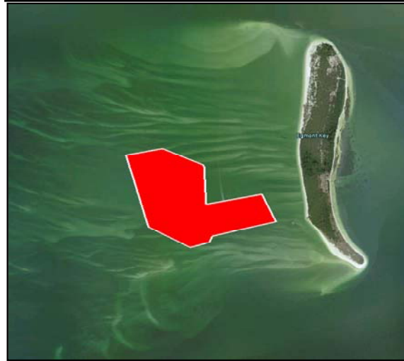
Figure 5. Nearshore berm placement planned for offshore of Egmont Key, Florida. Note that the shape of the placement area reflects cultural resource zoning due to the presence of a 19 th century era fort.
