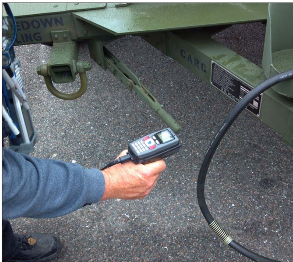
Figure 2: Electronic Scanner Being Used to Read a Data Plate with an IUID Data Matrix
