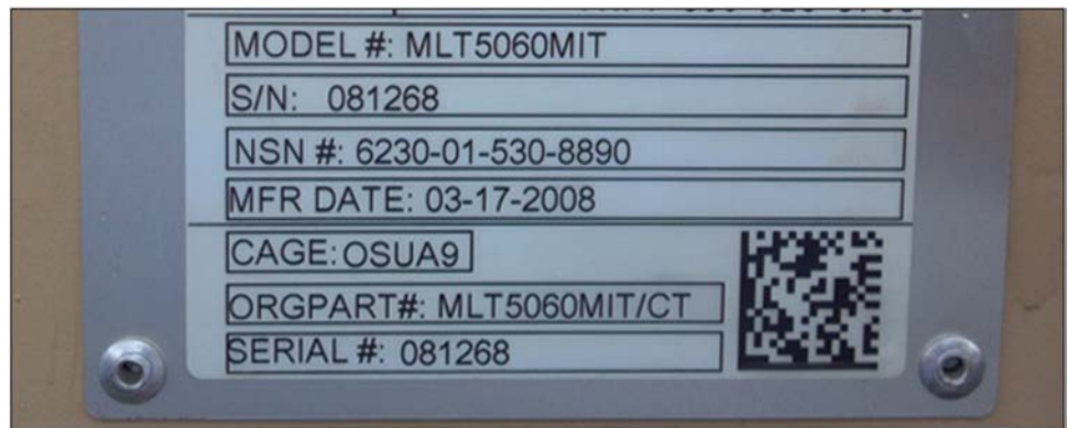
Figure 1: Data Plate with IUID Data Matrix
