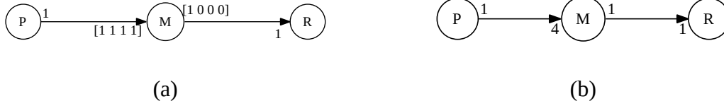
Figure 2.2: An application graph with a simple decimator actor M using the (a) CSDF, and (b) SDF models. Actor M is a decimator with a decimation factor of 4.
