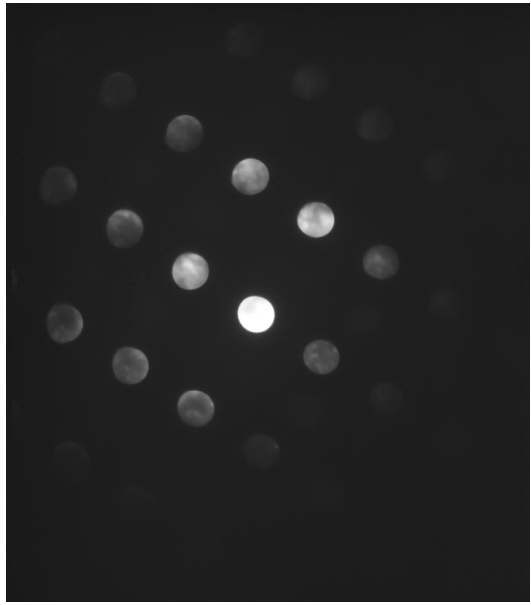
Figure 36: (a) TEM micrograph of sample taken at 6mm from UIT surface for Custom 465 aged at 950°F (b) &(c) SADP of image in figure 35 and 36a (d) Micro diffraction of image in figure 35b – UIT treated
