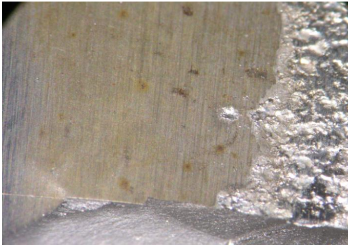
Figure 66 4340+ESD enlarged view of previous image showing multiple fatigue initiation sites from ESD deposit
