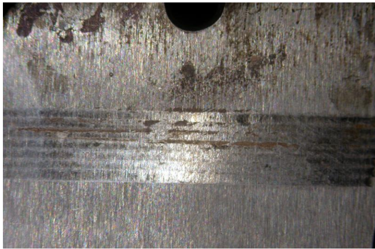
Figure 62 UIT treatment on both sample sides at radius to clamped wide shoulder
