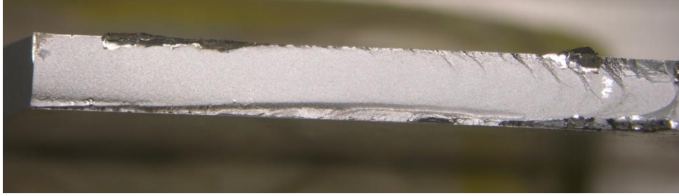
Figure 63 4340 baseline fatigue sample, 200ksi max stress, 72,000 cycle life
