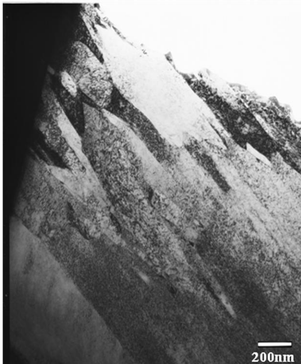
Figure 121: TEM micrograph of carbide precipitates in base material Ferrium S-53 alloy tempered at 934°F and 900°F – no ESD/ UIT treatment
