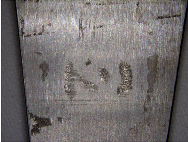
Figure 70 4340+ESD+UIT, surface ground after UIT revealing incomplete ESD fill areas
