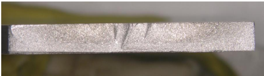
Figure 74 C465 aged at 1000°F, ESD+UIT, top view showing incomplete ESD fill after surface grinding flush with base sample. Cracking started at left, right, and middle incomplete fill areas
