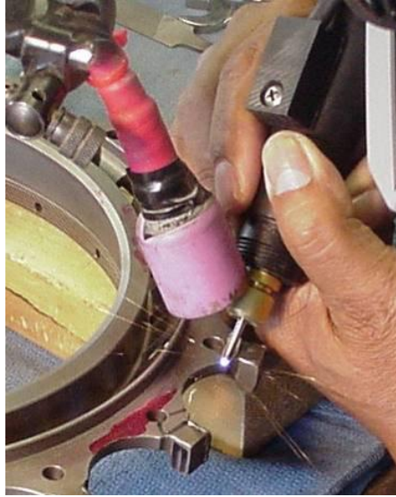
Figure 3: Manual ESD operation Gas cup provides electrode and deposit shielding [9]
