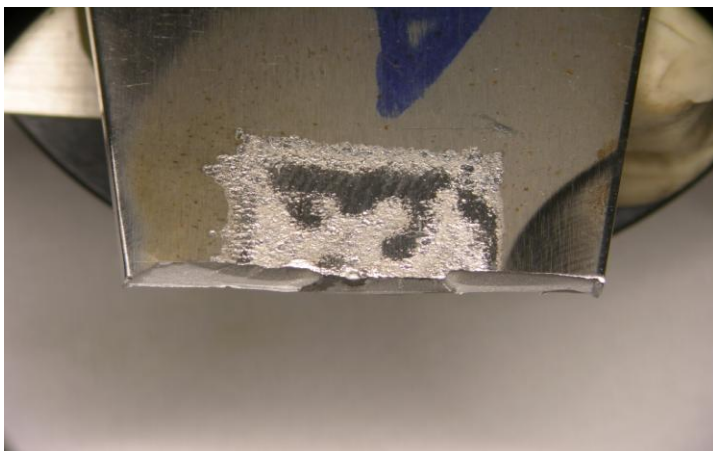
Figure 68 4340+ESD, top surface surface ground after ESD; ESD fill incomplete
