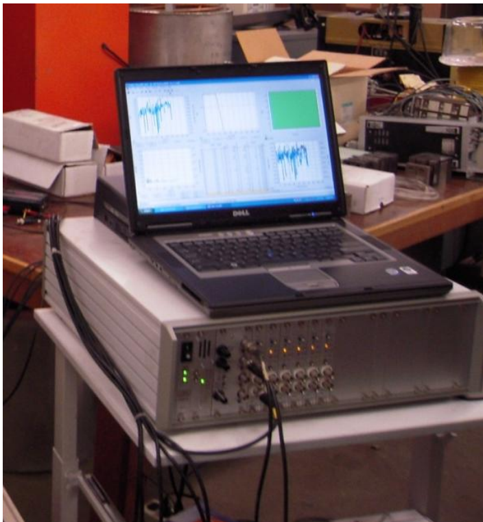
Figure 3, Rising Step load E399 test sample with acoustic emission sensor attached; Vallen multichannel AE AMSY5 system
