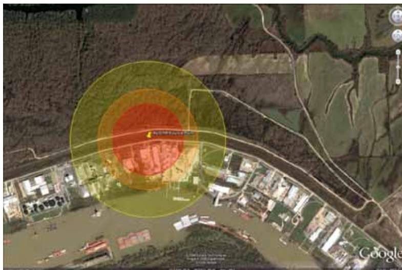
Figure 15. Release modeling of an explosion of a propylene tank for Test 2.
