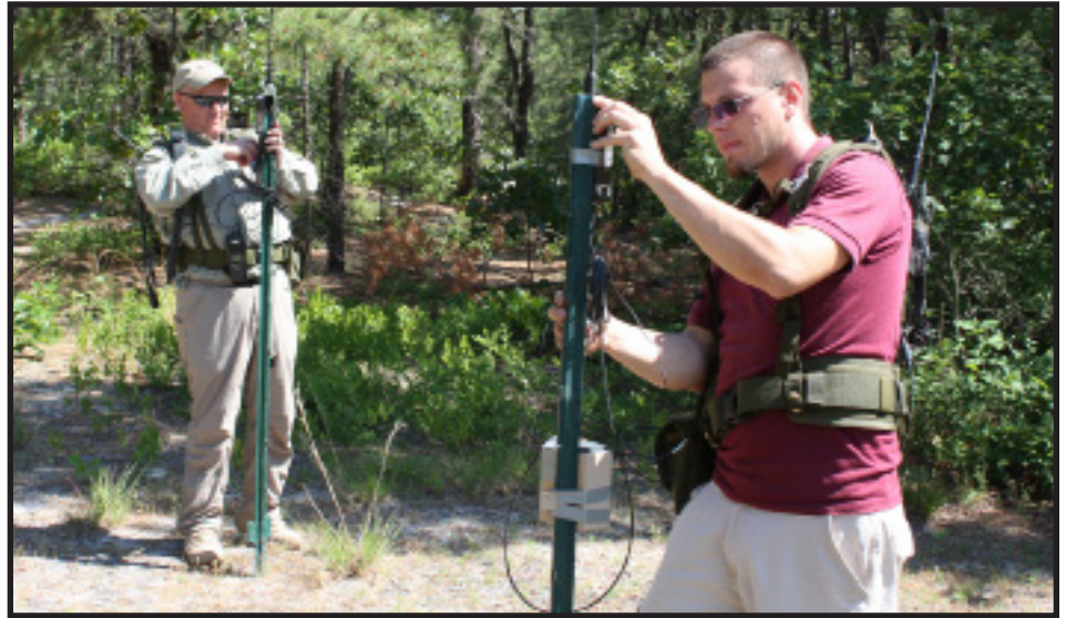
Rodney Smith (left), and Ted Krainski of C4ISR OTM set up radios as static nodes, representing stationary Soldiers. Live dismounts in the field interacted with the stationary nodes, passing scripted voice and situational awareness traffic from the squad leader down to the lowest level rifleman.
