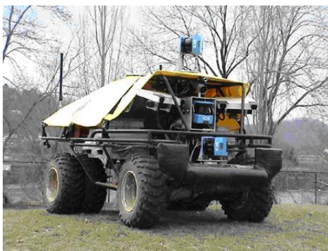
Figure 1.5.1: PerceptOR robot. A preliminary version of our results was verified on PerceptOR vehicles, designed to navigate in natural environments.
