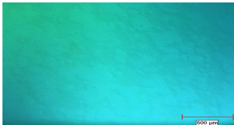
Figure 2-12. DIC image of an HLED sample after 24hrs exposure to ambient conditions.
