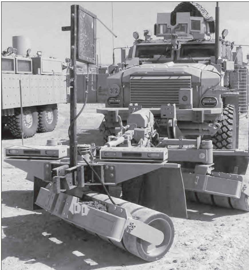
This U.S. Army Panther MMPV is equipped with a mine/IED roller to help neutralize or defeat explosive hazards.
