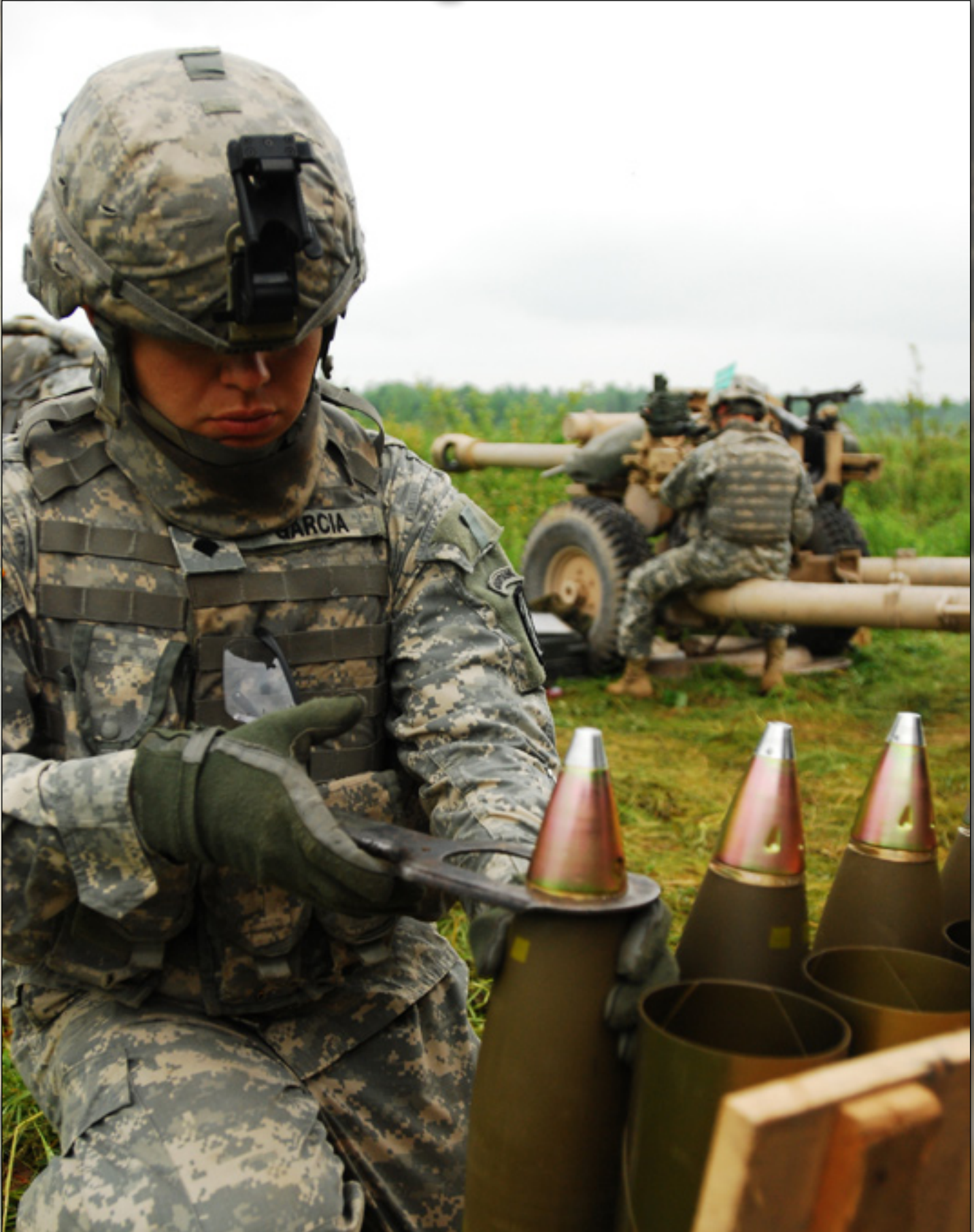
SPC Carlos Garcia of A Battery, 3rd Battalion, 6th Field Artillery, 10th Mountain Division, 1st Brigade Combat Team, prepares to install a fuse on an artillery round during a combined live-fire exercise at Fort Drum, N.Y., June 3, 2009 (Photo by SSG John P. Queen, U.S. Army)
