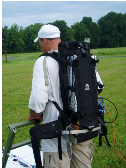
Figure 5-2 – TEMTADS 2x2 Electronics Backpack
