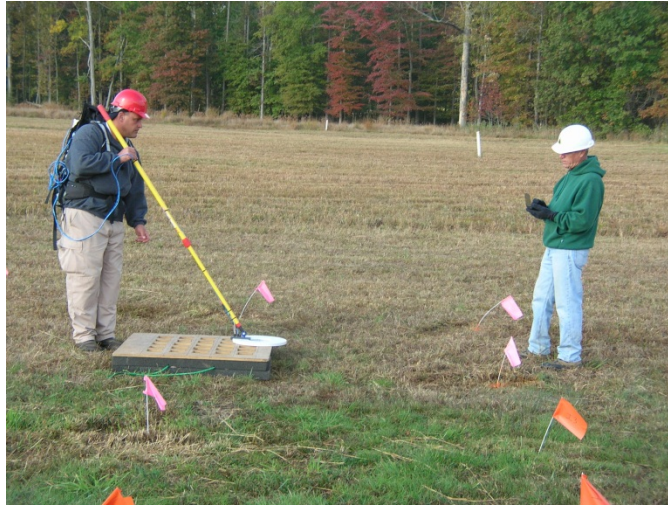
Figure 2-5 – The NRL TEMTADS Hand-Held Sensor
