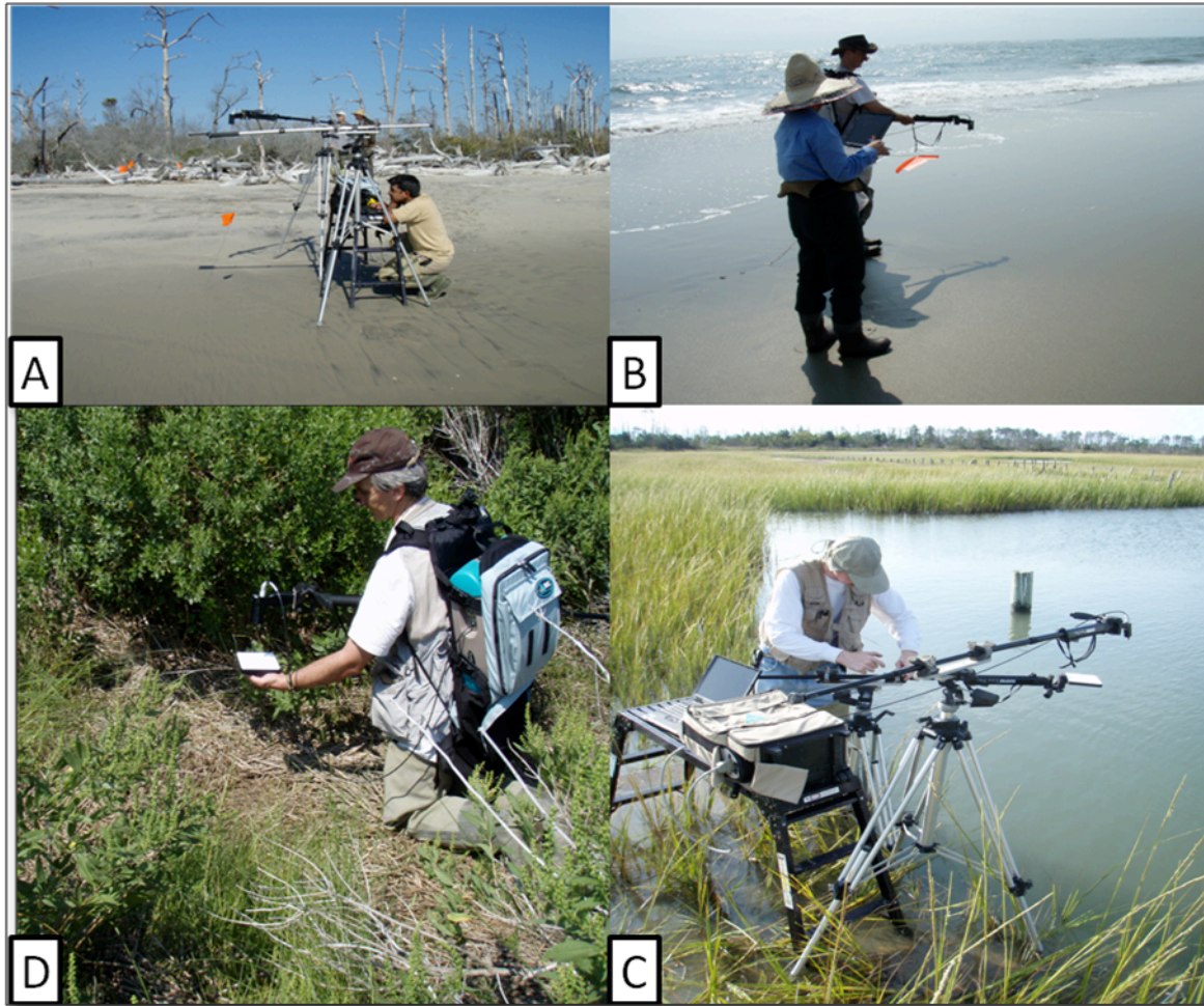
Figure 3.1. Spectra collection configurations. (A) Site spectra collection using two tripods. (B) Site spectra collection using one ASD and hand-held Spectralon® plaque. (C) Shallow water bathymetry collection using two tripods. (D) In situ vegetation collection using one ASD and handheld Spectralon® plaque.
