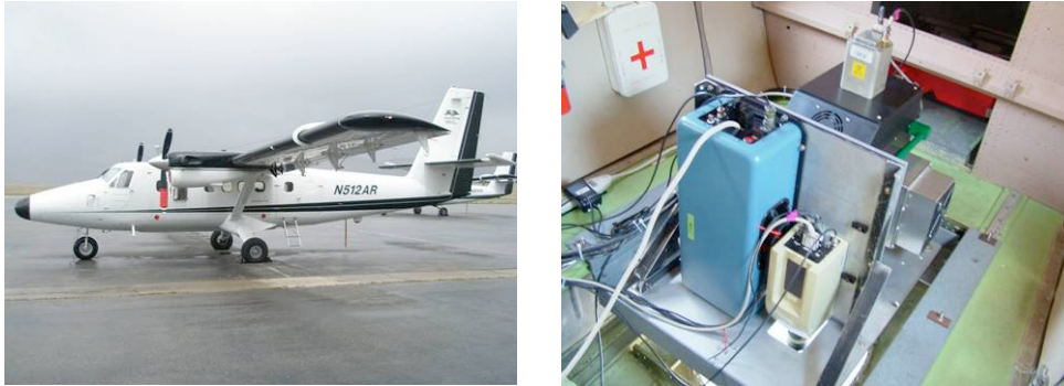
Figure 1.3. VCR'07 platforms and sensors. The left panel is the Twin Otter aircraft used to support remote sensing over Cape Charles, VA. The right panel is the NRL CASI-1500 VNIR hyperspectral sensor, Surface Optics SOC-700-SW SWIR hyperspectral sensor, and single channel mid-wave infra-red camera onboard the twin otter. ONR provided platform support and data was collected simultaneously from all three sensors throughout VCR'07.
