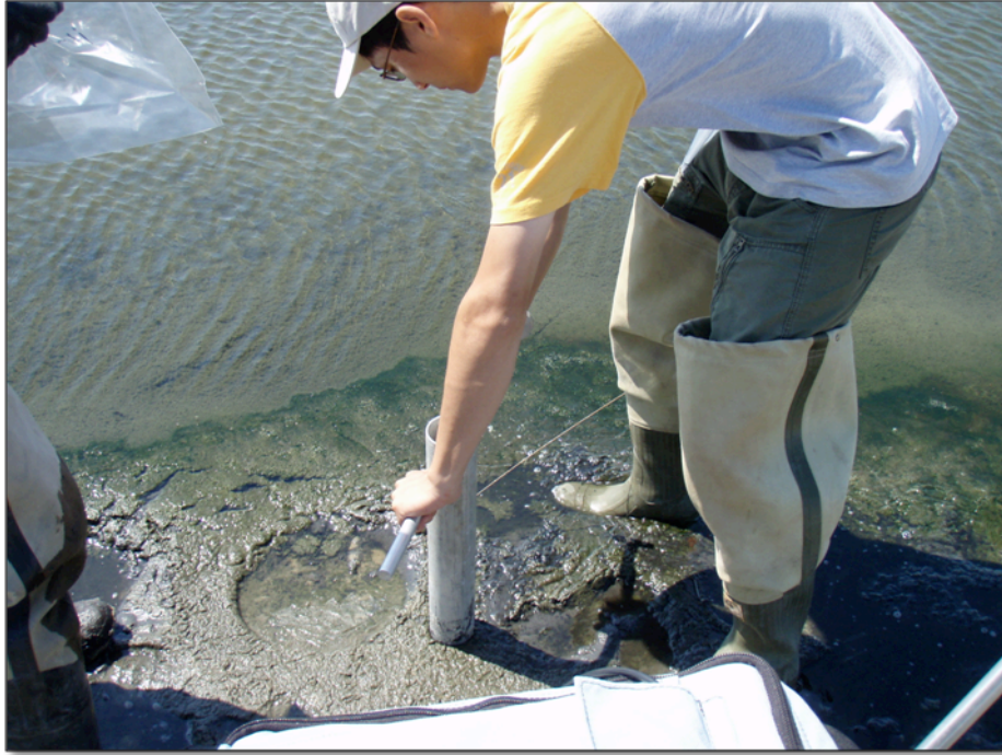
Figure 3.6. Grab sampler in use extracting core sample.
