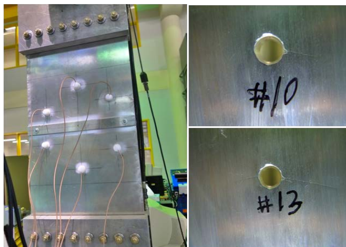
Figure 3.7. Plate #8 with bonded doubler, central drilled through-hole, and side through-holes with bolts installed.
