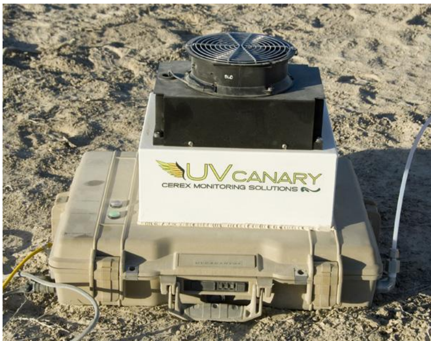
UV Canary system set up for real-time chlorine gas detection
