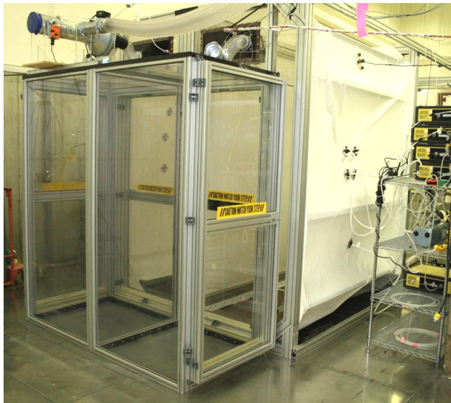
Airlocks attached to Novel Closures Test Fixture
