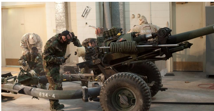
CBR contamination survivability test
