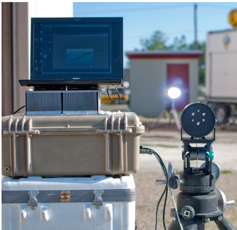
UV Sentry open-path spectrometer
