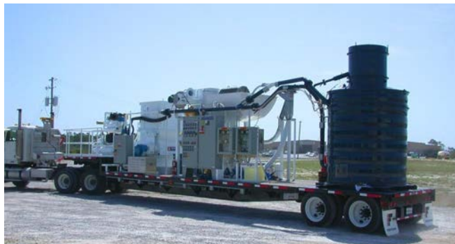
Figure 1: TWES Trailer #1 with solid fuel handling equipment; the furnace has been move to Trailer #2.
