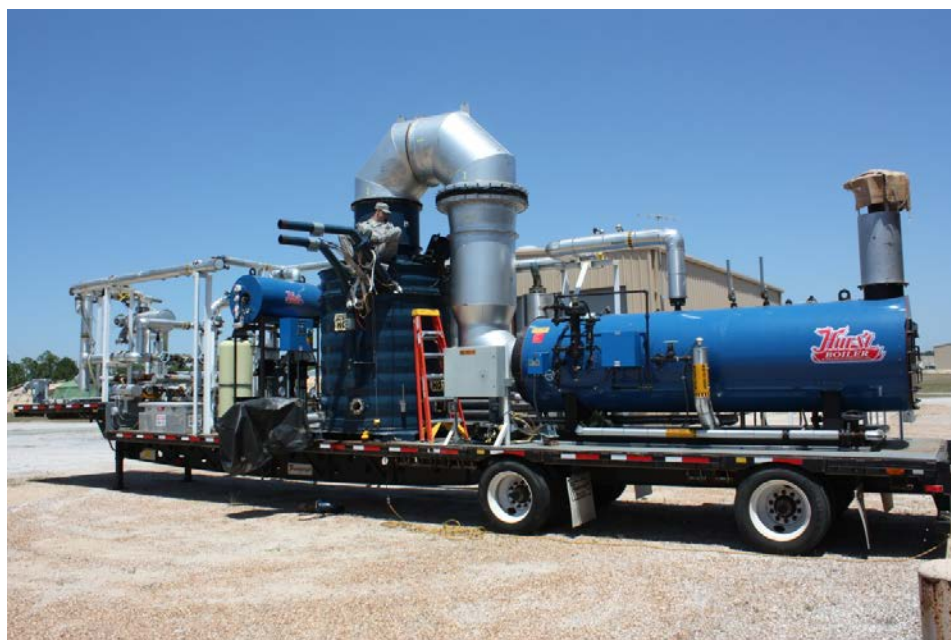
Figure 2: TWES Trailer #2 with steam generation equipment attached to furnace; The HRSG is on the aft end of the trailer.
