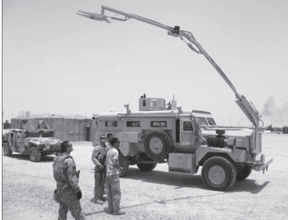
Soldiers from the 1st Cavalry Division train soldiers from the 14th Field Engineers Regiment to operate the interrogator arms of their light armored vehicles.
