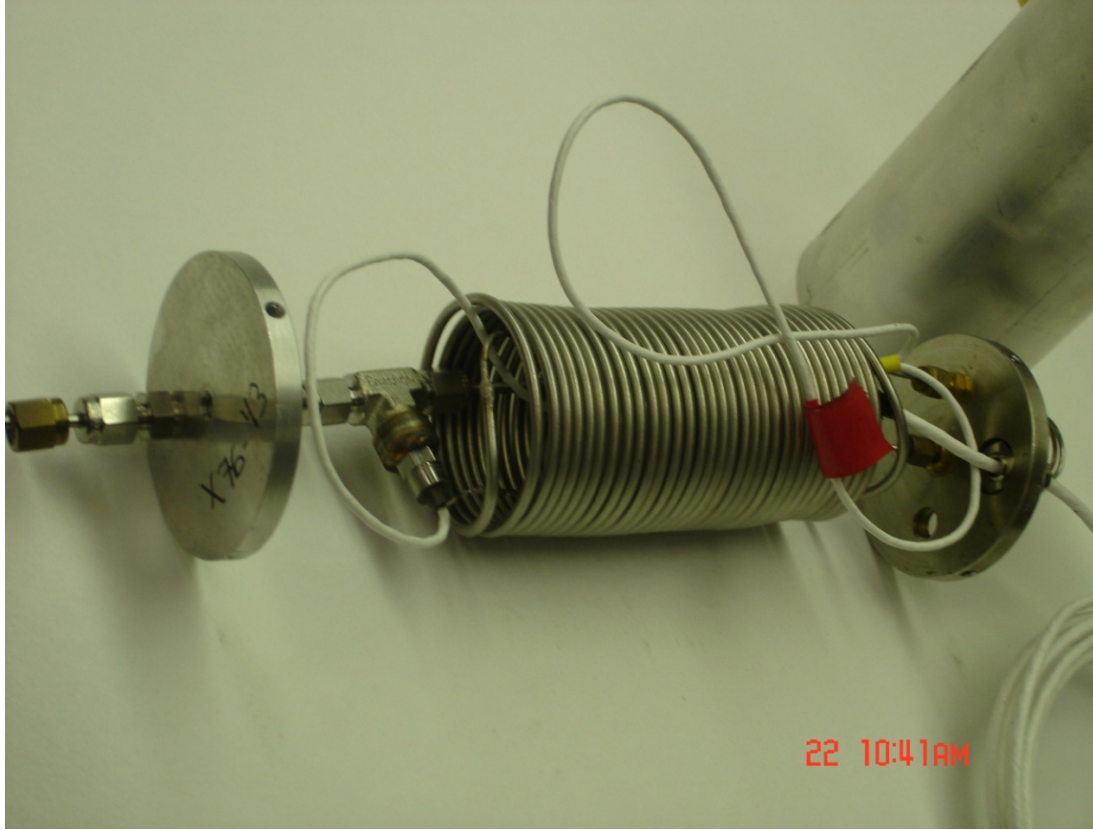
Figure 4. Schematic and photograph of Semi-Infinite Transducers (SITs).
