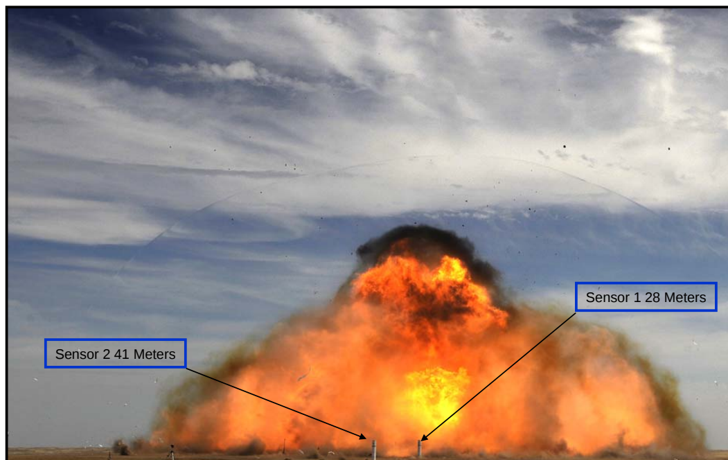
Figure 6b, fireball of actual event with four color IR gages fielded.
