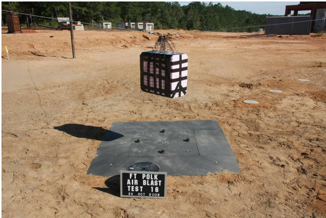
Figure 2. Charge orientation for a box-shaped explosive charge.
