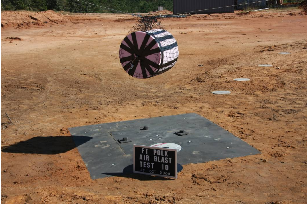
Figure 1. Charge and gage layout for a cylindrical explosive charge.
