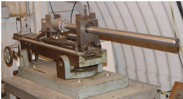
Figure 5: Modern Bond Universal Small-Arms Receiver Used to Fire the Projectiles
