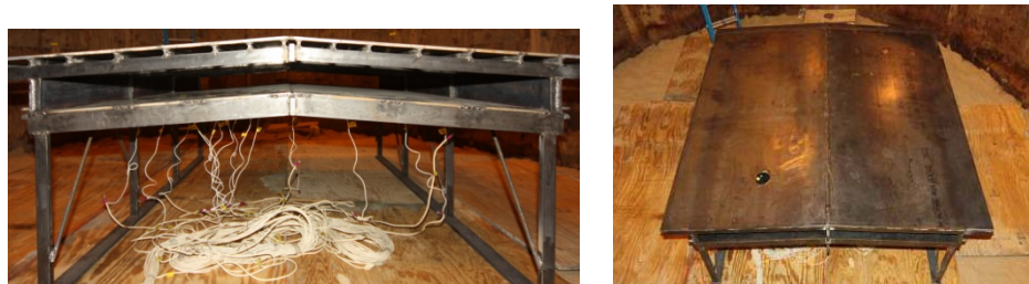
Figure 3. Elevation and Plan View of Instrumented Scale Model, Showing a Scaled 3-ft Opening.
