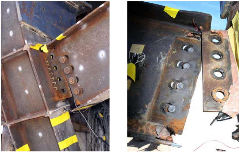
Figure 4. Traditional Seismic Moment (WUF) Connection at Ultimate Failure (5)
