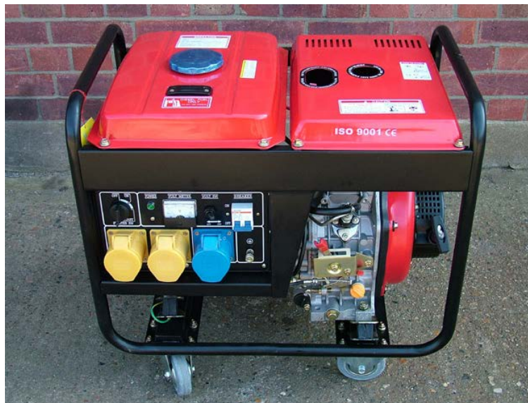
Figure 6. Typical Portable Diesel Generator (From: Dobler, 2008)
