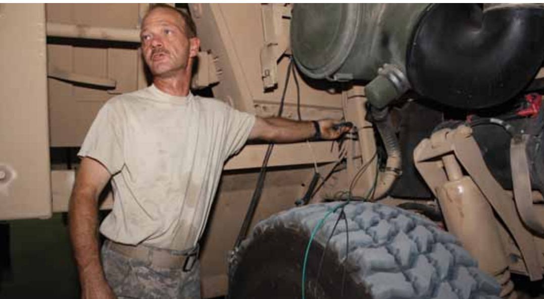
A 416th Transportation Company Soldier rewires a Caiman Plus mine-resistant ambush-protected vehicle in the exchange shop. (Photo by SGT Refugio Medina, 416th Transportation Company)
