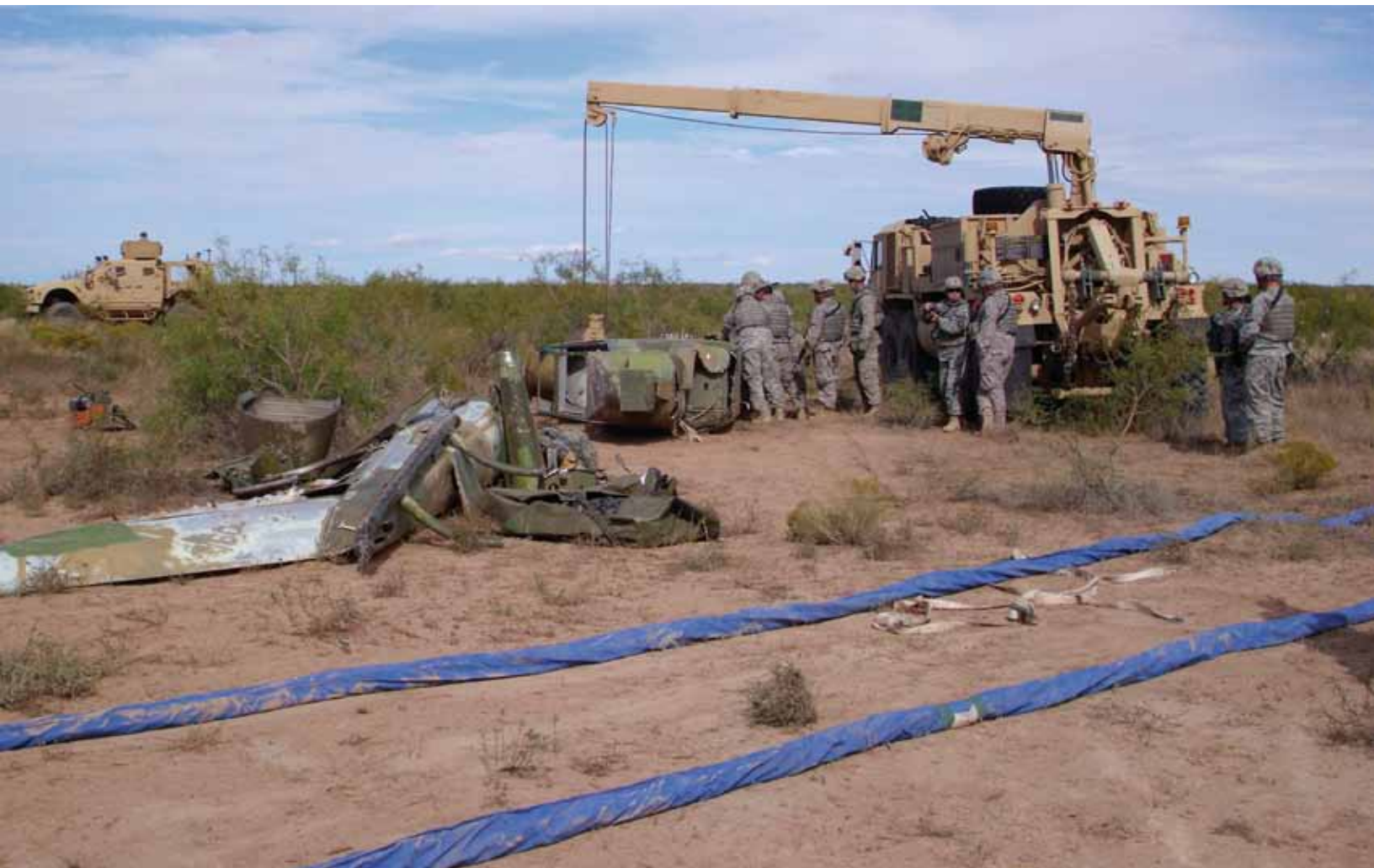
Above, Soldiers from A Company, 563d Aviation Support Battalion, receive a convoy commander's briefing before departing on a mission. Below, 563d Aviation Support Battalion Soldiers use the crane on a heavy expanded-mobility tactical truck wrecker during a downed aircraft recovery team exercise.
