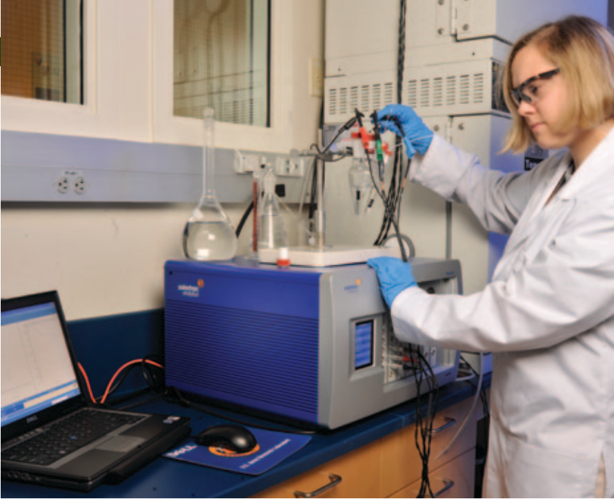
Michelle Marx analyzing impedance spectra from high power Li-ion batteries.
