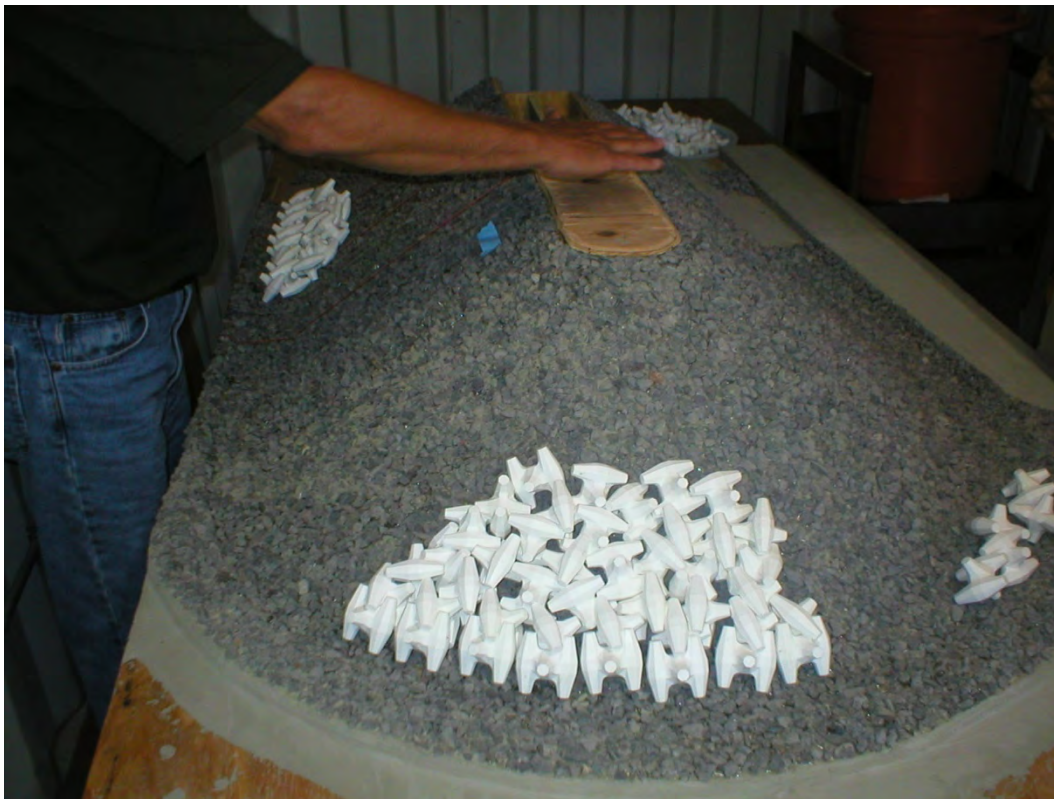
Figure 3.2. Contractor scale-model of Kaumalapau Harbor breakwater and Core-Loc armor units.
