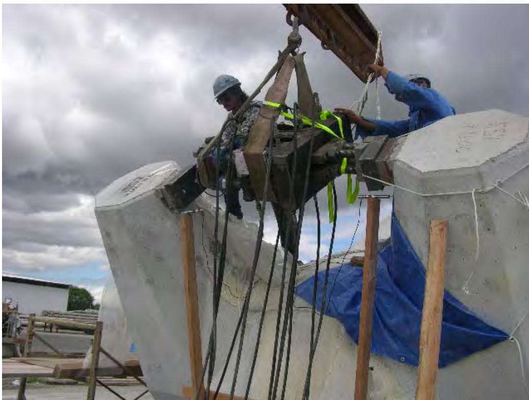
Figure 5.7. Hydraulic ram placed between the Core-Loc legs (O'Neil and Haskins 2008).
