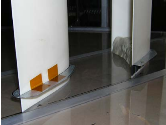
Figure 9. Image of cascade airfoils with fence and pressure surface modifications
