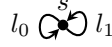
Figure 6. s is not bisimilar with itself among the overlying \{l_0, l_1\} -labelled execution system whose executions correspond to all infinite paths in the diagram, and that whose executions correspond to the infinite paths that go through each of the two loops infinitely often.
