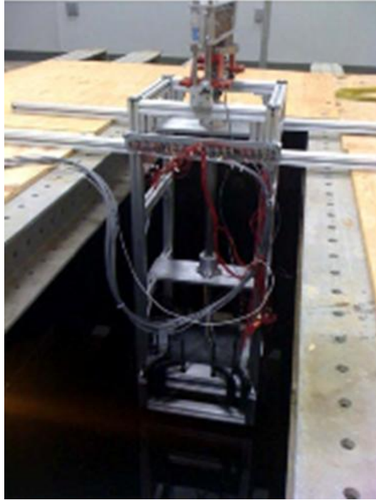
Figure 17. Impact test machine lowered into the test tank (From [13])
