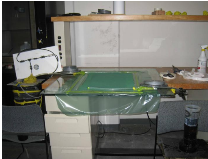
Figure 6. VARTM setup in the laboratory
