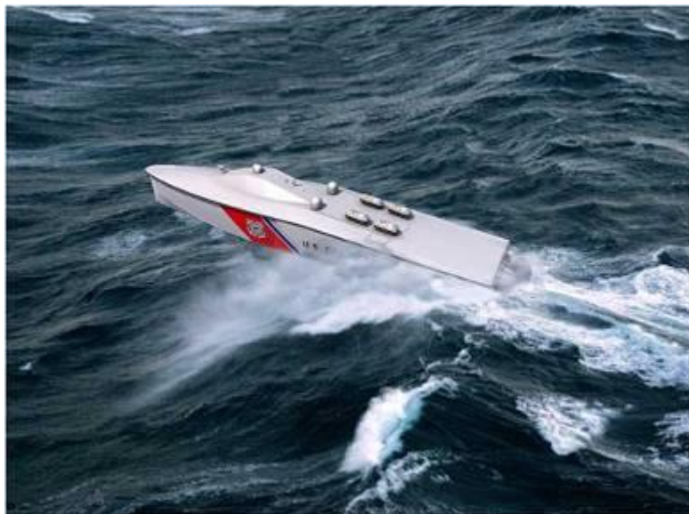
Figure 2. USV built from nanotube-reinforced carbon fiber composites. (From [2])
