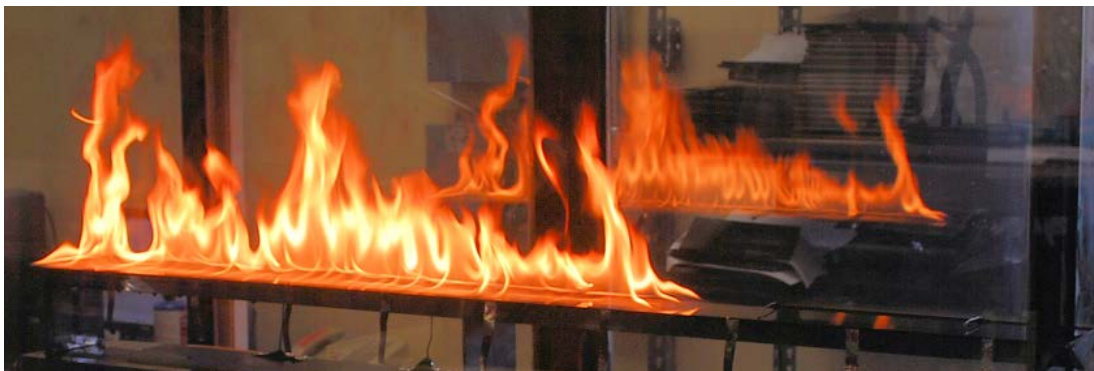
Figure 4. Flame Speed Propagation Test in Progress
