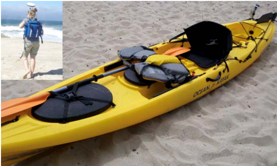
Figure 7. Sea kayak with echo sounder and Ashtech z-Xtreme GPS attached. An Ashtech z-Xtreme GPS mounted in a backpack used for beach surveys.
