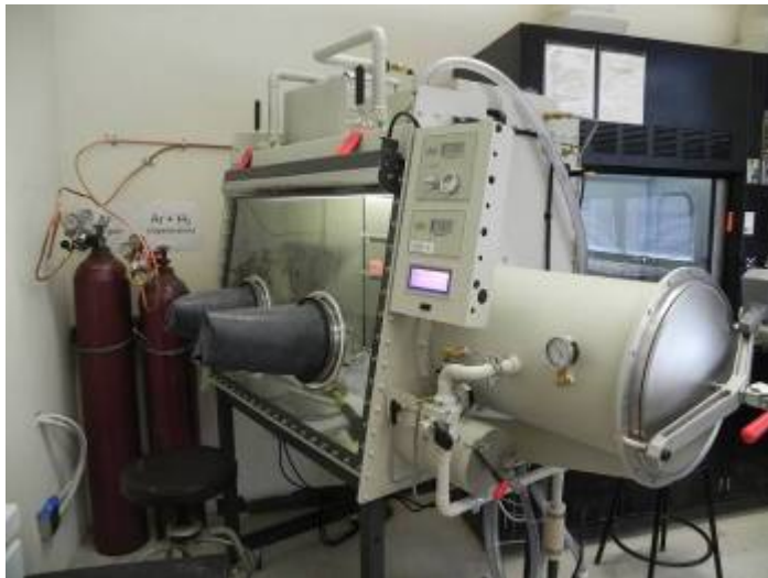
Figure 14. An Argon-filled glove box used for battery assembly. The glove box prevents moisture and oxygen from interacting with the internal battery components and reducing the cycle life of the battery (From [15]).
