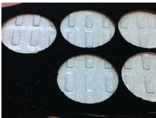
Figure 26. Damage to the electrode film using the MTI disc cutter was minimal.
