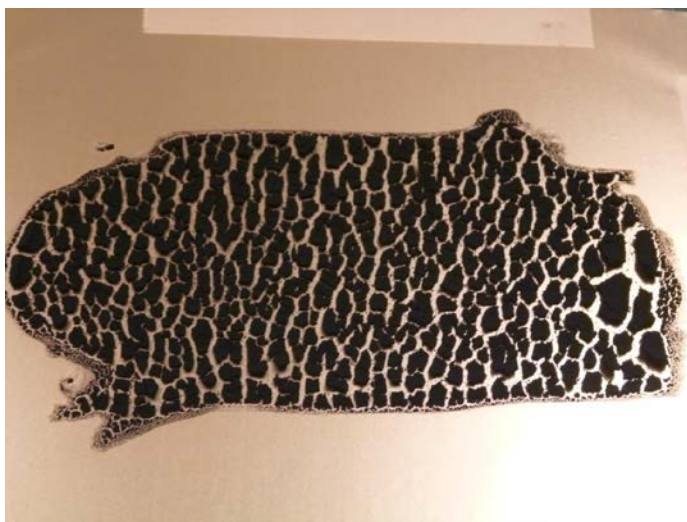
Figure 20. Cracking in MWCNT electrode film was consistently experienced in the fabrication process.
