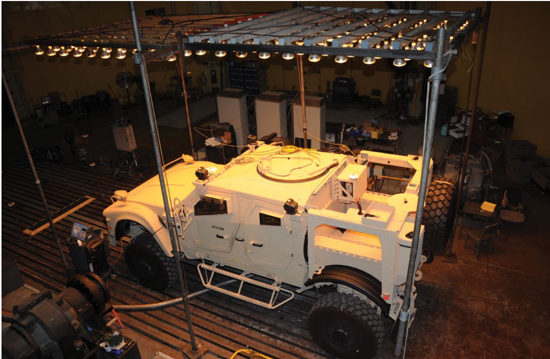
An MRAP is tested in TARDEC's full-load environmental testing chamber, which simulates extreme heat and wind conditions. As vehicles are tested in diverse climates, understanding how they react to heat, cold, wind and other conditions can help us keep them operating wherever Soldiers are needed. (U.S. Army TARDEC photo.)
