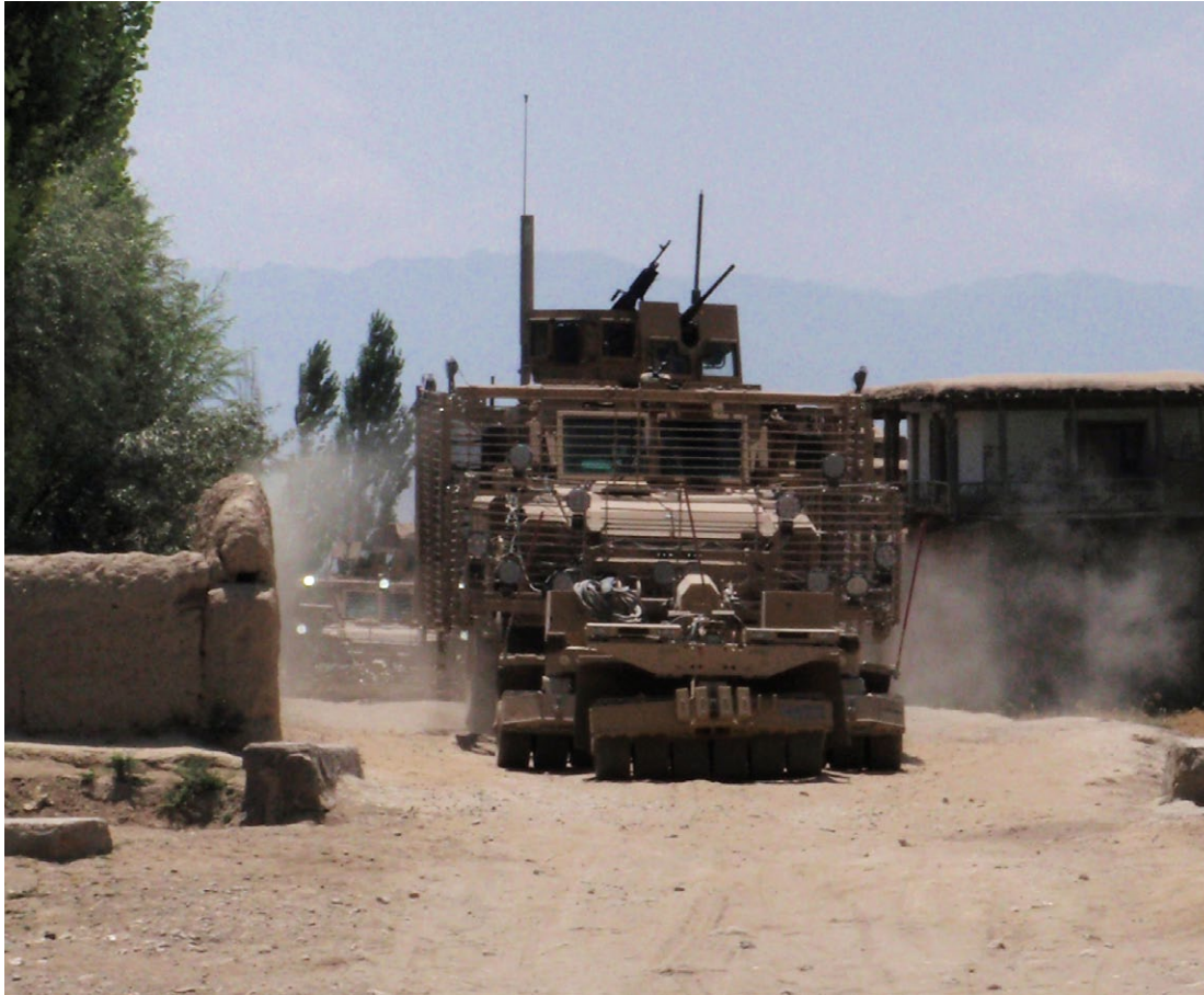
An MRAP crosses a dangerous bridge that is known for bomb detonation just outside of a village in Afghanistan. The MRAP is equipped with the SPARK mine roller and the Thrown Object Protection System, both designed by TARDEC engineers to protect Soldiers from threats in the field. (Photo by SPC Theodore Schmidt)
