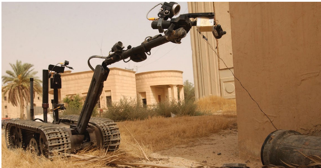
A TALON robot demonstrates its ability to destroy improvised explosive device firing units without subjecting Soldiers to danger. Unmanned ground vehicles have been critical in keeping our Soldiers out of harm's way and putting distance between them and threats. (U.S. Army photo.)
