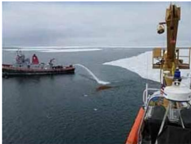
Figure 15. Fire monitor water cannon on stern of T/V Erika Kobasic herding ice and oil surrogates toward collection pocket created by CGC Hollyhock and edge of ice sheet.
