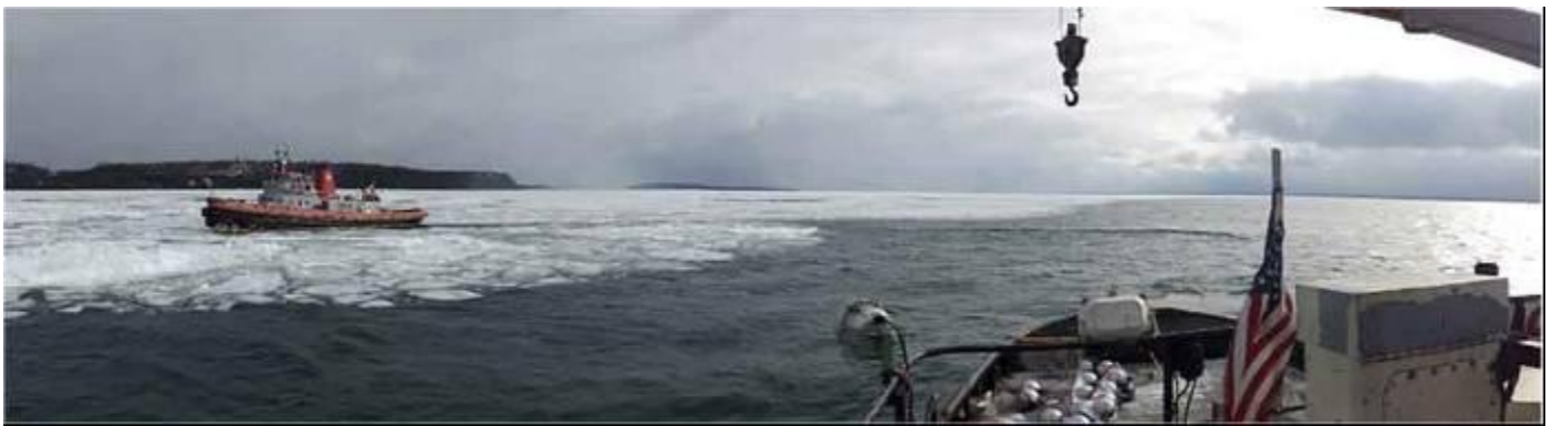
Figure 19. PyroBoom deployed and towed by two tugboats to simulate collection of oil in rubble ice.
