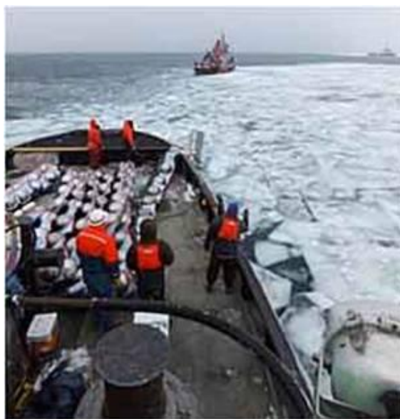
Figure 16. PyroBoom in process of being deployed in rubble ice from stern of tugboat.
