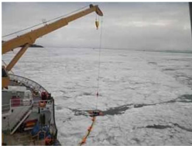
Figure 5. Helix skimmer deployed in open water pocket using 'whip' crane.
