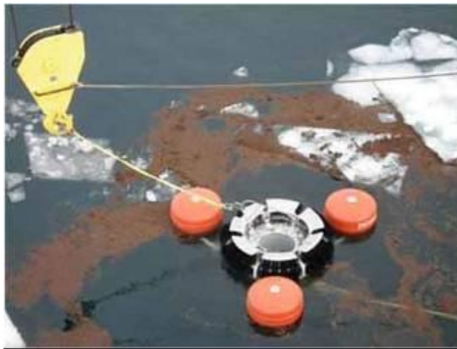
Figure 11. Details of Helix skimmer in process of recovering peat moss oil spill surrogate.
