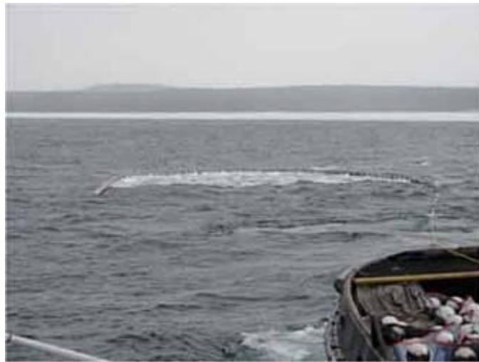
Figure 20. Towing the PyroBoom in a 'U'-shaped configuration with captured ice.
