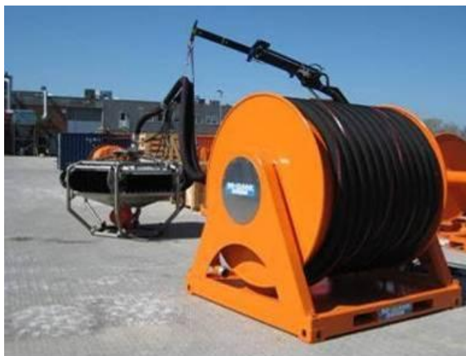
Figure A-9. Polar Bear skimmer (left) and associated reel with crane (right).
