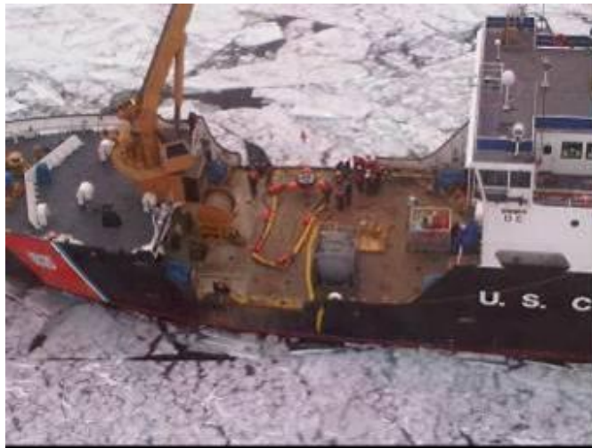
Figure 7. A temporary storage container (gray tank) mid-deck on a Juniper Class Seagoing WLB.
