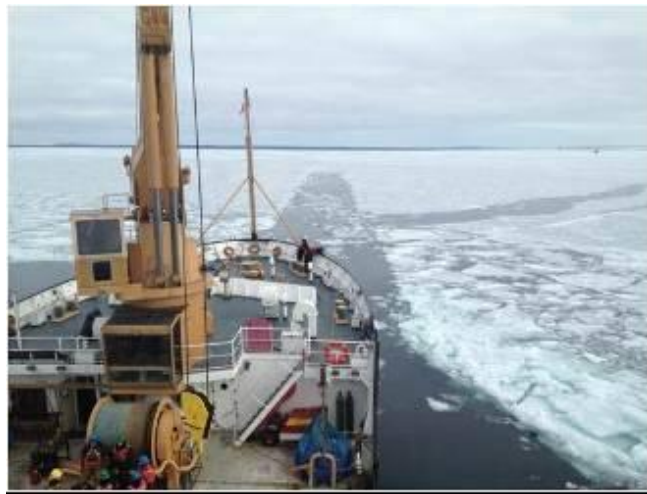
Figure 8. Channel or 'slot' created in sheet ice by CGC Hollyhock to facilitate oil skimmer deployment.
