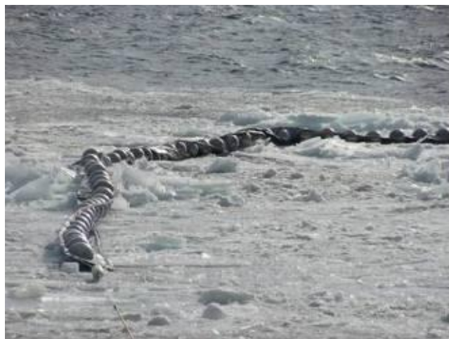
Figure 17. PyroBoom surrounding selected rubble ice volume.
