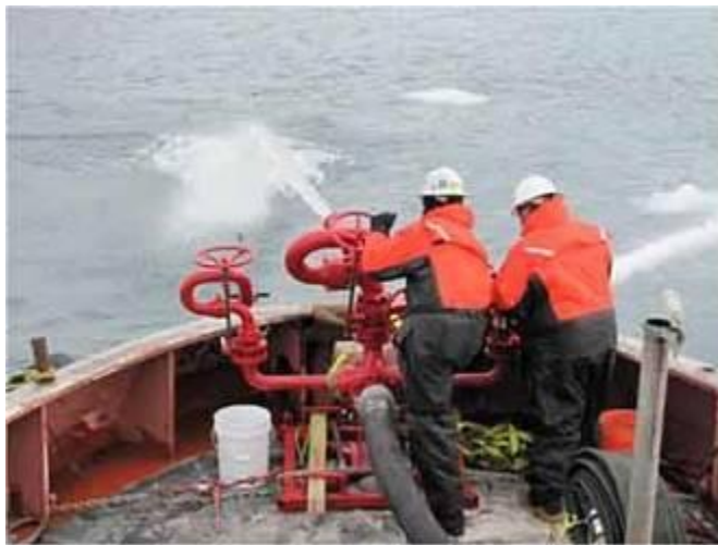
Figure 13. Stern-mounted fire monitor water cannon on T/V Erika Kobasic demonstrating herding ice and oil surrogate.
