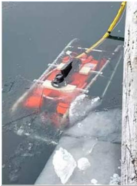
Figure 34. ROV deployed from T/V Nickelena in water pocket near ice sheet edge.
