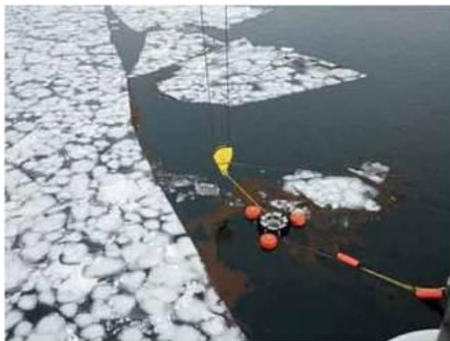
Figure 10. Helix skimmer deployed near ice edge by crane using 750-lb block; peat moss oil spill surrogate can be seen surrounding skimmer brushes.
