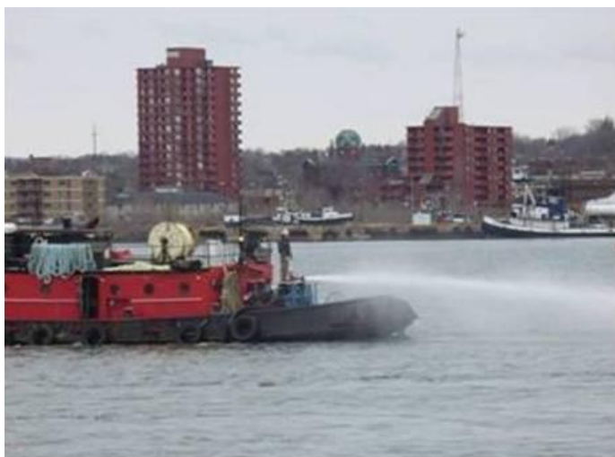
Figure G-3. Open water – herding: apparatus mounted on a tugboat.
