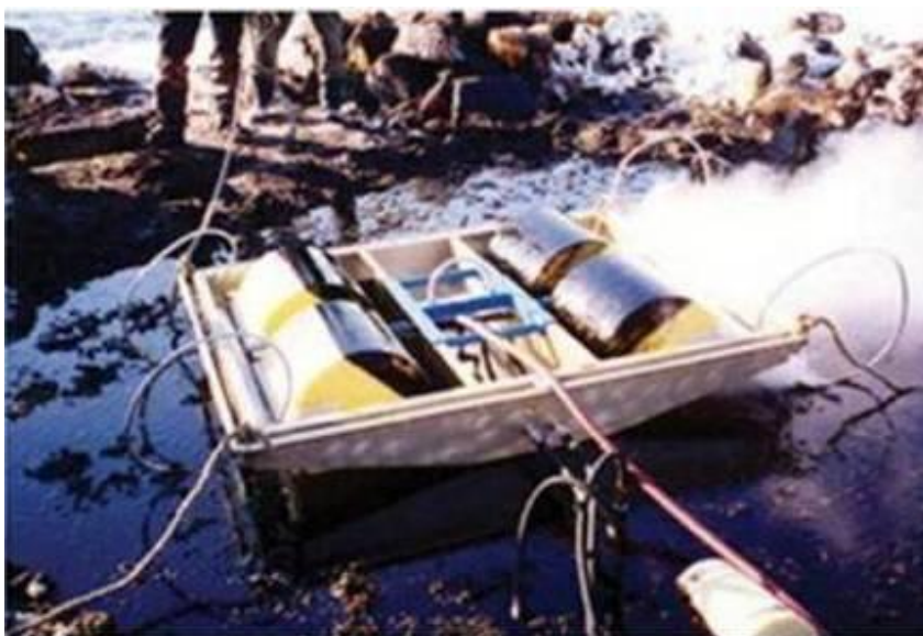
Figure A-5. Steam-heated drum skimmer.
