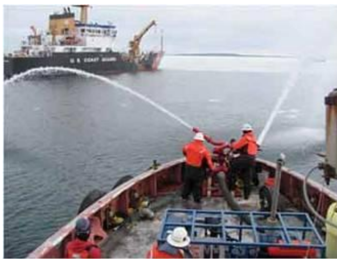
Figure 14. Two fire monitor water cannons on stern of T/V Erika Kobasic herding ice towards pocket in sheet ice created by CGC Hollyhock.
