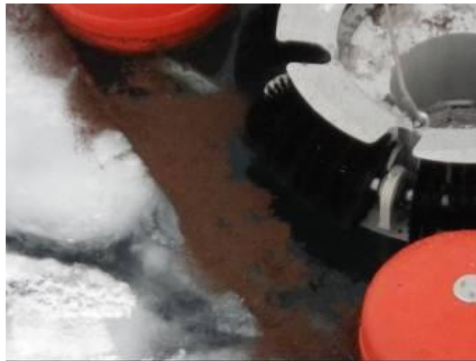
Figure 12. Extreme close-up of skimmer in operation near an ice edge, showing adjacent and collected peat moss, small bits of collected ice, and minimal collected liquid water.
