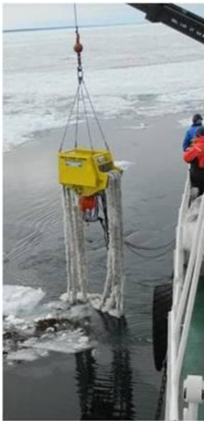
Figure 31. Rope mop skimmer deployed in open water pocket from T/V Reliance on Day 2 of the demonstration.
