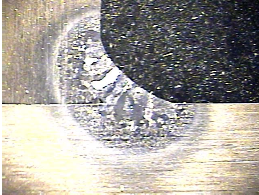
Figure 15 HAZ shown in this TIG weld macrograph
