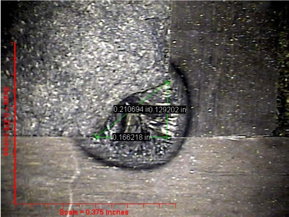
Figure 3 MIG titanium weld displays measuring standards
