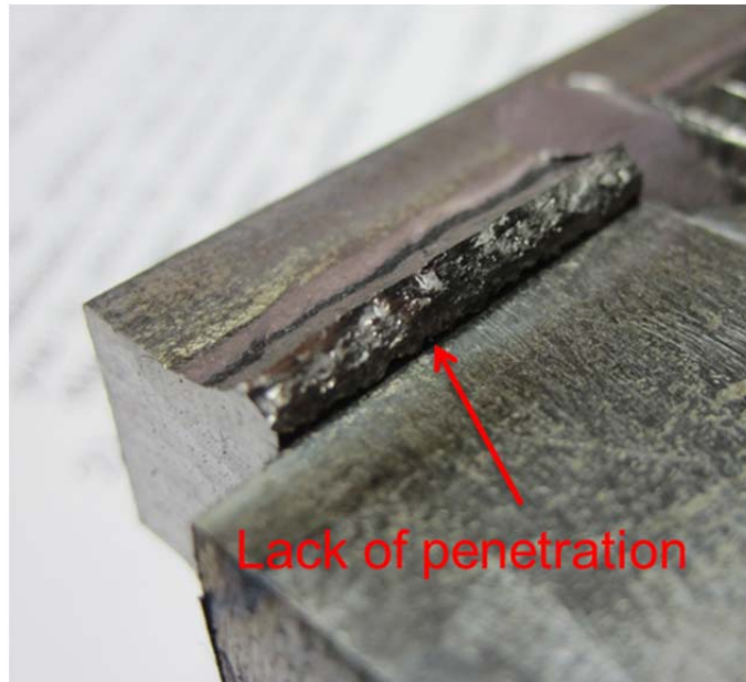
Figure 50 Another example of the recurrent lack of penetration
