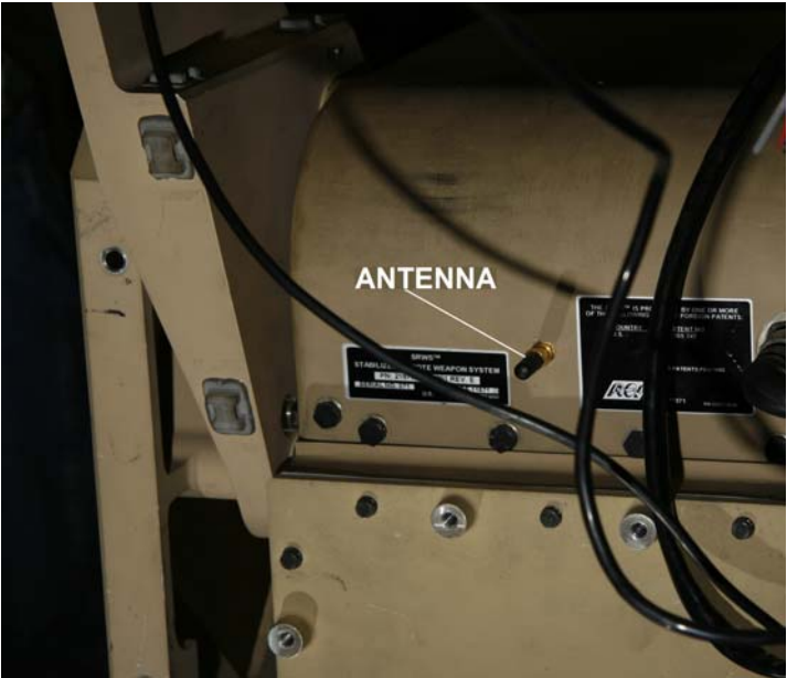
Fig. 14. External WSN antenna mounted on the outside of the closed chassis.
