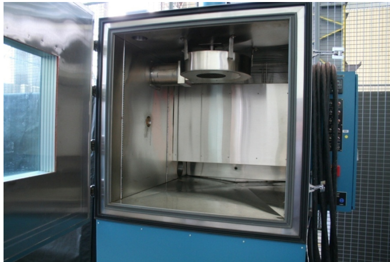
Figure 6: Cincinnati Sub-Zero (CSZ) Chamber for Controlling Test Environment
