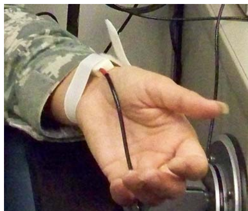
Figure 5. Correct placement of the radial artery reference sensor.
